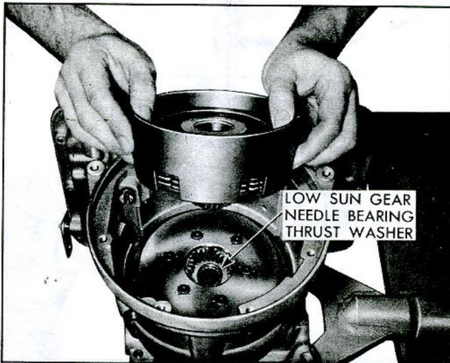
Fig. 7E-23—Removing Clutch Drum
