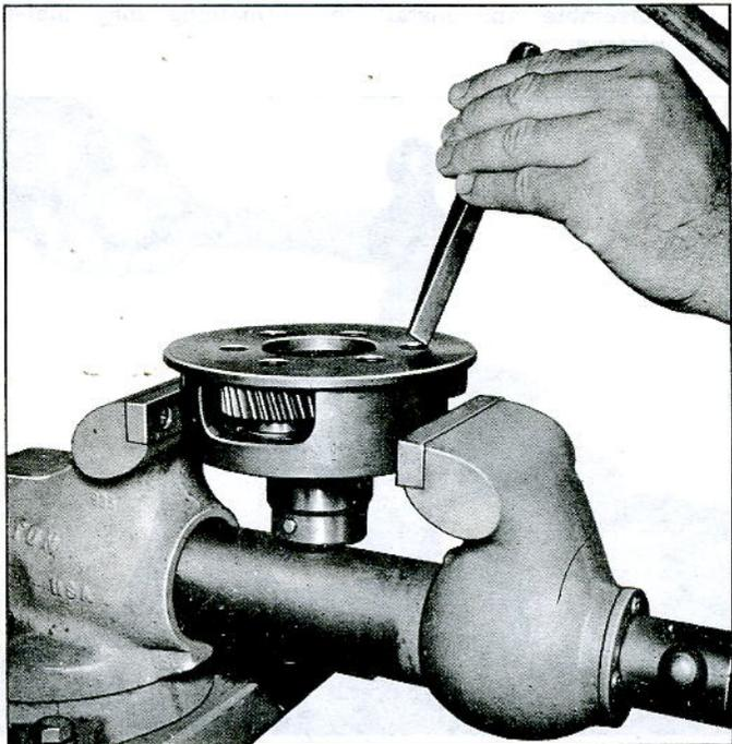
Fig. 7E-48—Staking Planet Pinion Shaft
