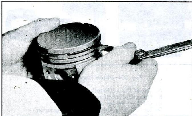
Fig. 106—Measuring Ring Groove Clearance
