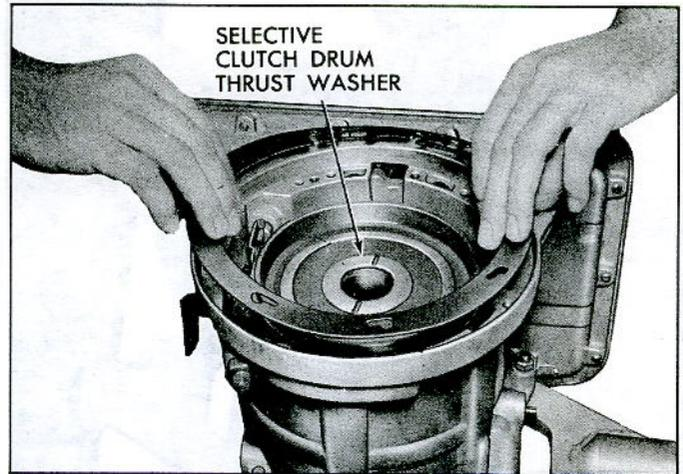
Fig. 7E-57—Installing Front Pump Gasket
