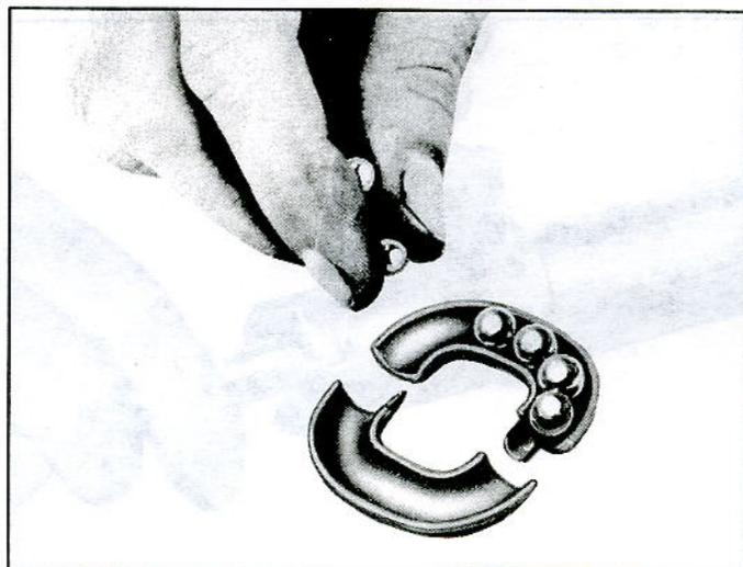
Fig. 14—Filling Ball Guides
