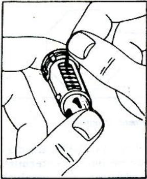
Fig. 14—Inserting Tumbler Springs
