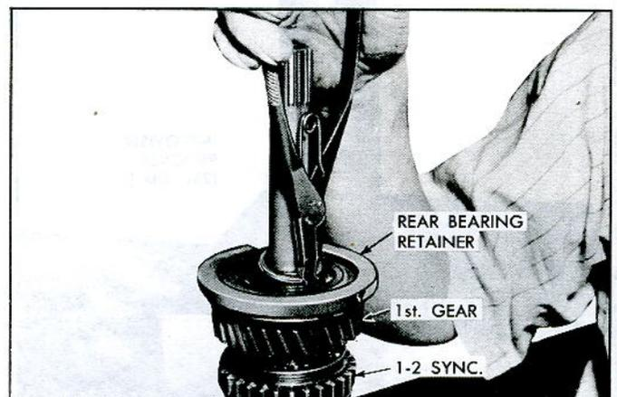
Fig. 7B-10—Rear Bearing Snap Ring
