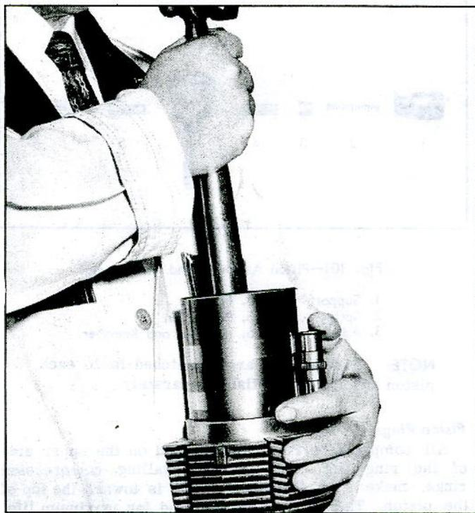
Fig. 107—Installing Piston in Cylinder
