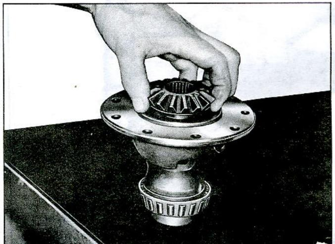
Fig. 32—Installing Side Gear in Differential Case
