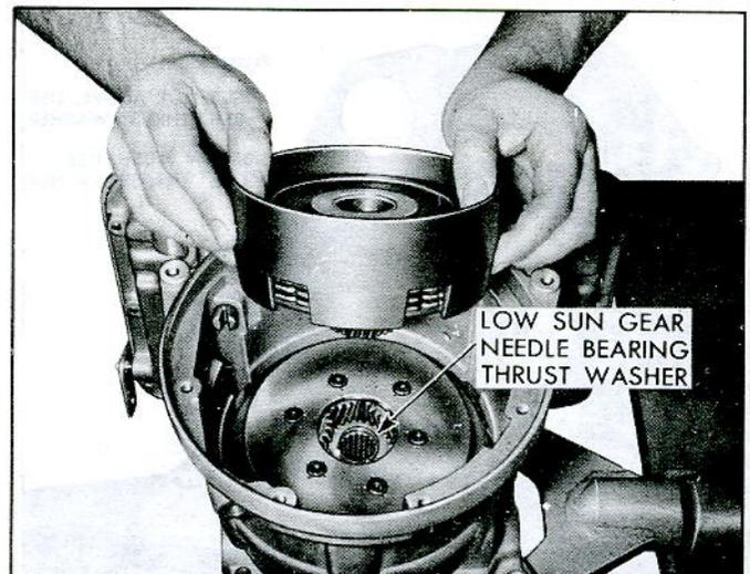
Fig. 7E-54—Installing Clutch Drum
