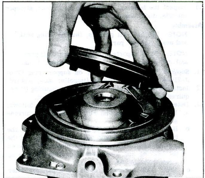
Fig. 48—Heat Shield Spring Ring Installation
