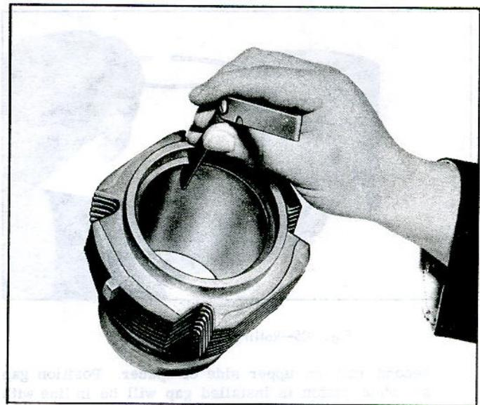
Fig. 103—Measuring Ring Gap
