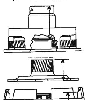
The top drawing is the Planetary Gear Assy. which is measured from the Thrust Washer (in cutaway) to the top of the collar. The measurements were:
