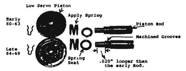
Only the late has the machined grooves. I suppose the new rod has something to do with the shift timing.
