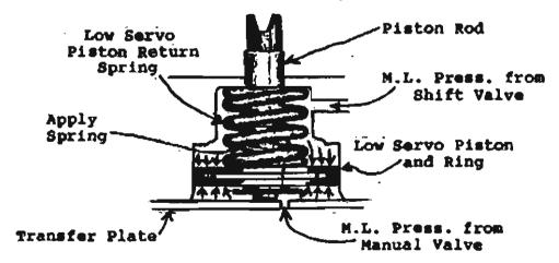
The sketch shows the piston with Main Line oil pressure on both sides of the piston, and the Piston Return Spring having
