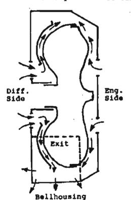
differential rebuilder breaks or leaves out this ring, the diff. will still work fine but now your PG will be at risk because of lack of pressure of the oil that is supposed to lubricate and cool the working parts of your PG. During normal operation any oil leaking past the ring will return to the sump.
