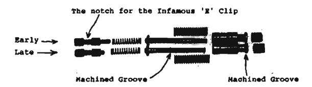
The reason the shaft was shortened was because if the early long shaft was used for the new adjustment, there would be a possibility that the end of the shaft might protrude past the end of the adjustable nut, and the required pressure drop would not be able to be obtained due to this obstruction.
