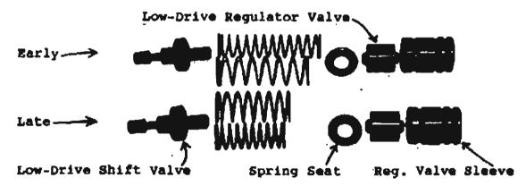
The longer pair of springs of the early shift valve are replaced by a shorter pair of springs, which take away PART of the advantage of the "Keep it in Low" gang. This however, is not enough to get the shift speed down within reason. (All the other parts of the Shift Valve remain the same for both early and late.)
