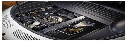
At least, not by American standards of 1963, which were a pledge of allegiance to the classic layout of liquid-cooled front-engine and gearbox and rear-wheel drive. The Testudo came with the Corvair high-performance 145 cubic-inch flat-six rear-mounted plant. It was small enough to allow Giugiaro to create his wonderful optical illusion but strong enough to push the car around without effort.
