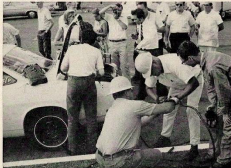
Air passing through wet seat cushions helped cool batteries. Typical scene at a recharging stop for the MIT Corvair team.
