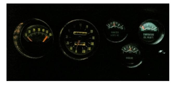
EM standard dashes can be updated also; all is the same as above. Remember the dash lights have a grey wire running to each bulb socket. The dimmer switch will not work with the LED's the will remain bright and turn off as the dimmer is turned.
