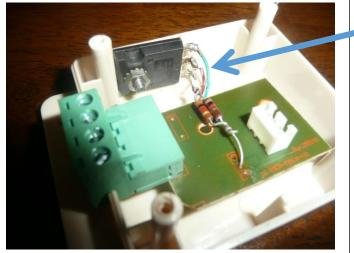
Caution red and green wires are reversed in this photo. Red wire should have been on the top.
