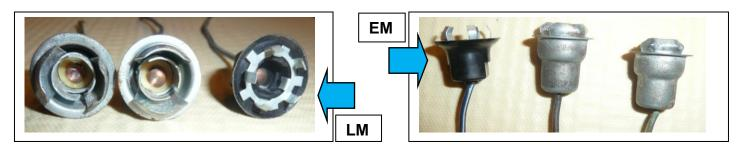
Replace the Late Model (LM) Corsa tack bulb sockets with the Early Model (EM) version.
