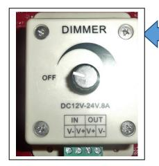
This is a Pulse Width Modulator type dimmer. It dims by sending pulses of varying width to the light source. It is efficient but may cause some noise in an AM or FM radio.
