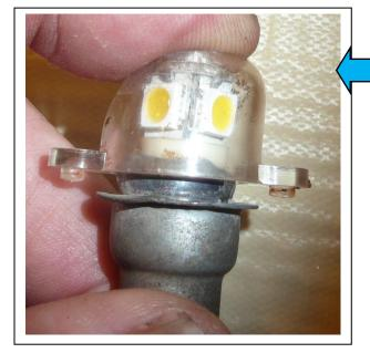
LED is too long and will not fit in Tack with plastic diffuser installed.
