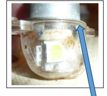
Insert the bulb in the socket with the flats aligned with the tab in the socket. The bulb should slide past the original stop position.
