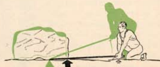
Smaller force moves greater distance.
