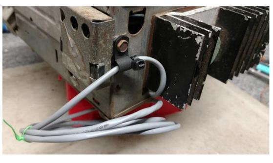
Tie strap the cables together (left picture) and re-mount the socket to the radio using the two screws.
