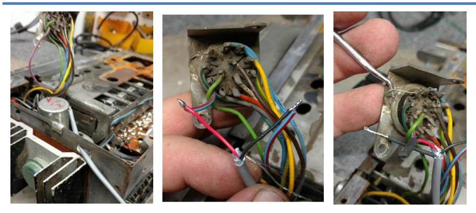
Run the cable into the radio near the heat sink like shown in the left picture.
