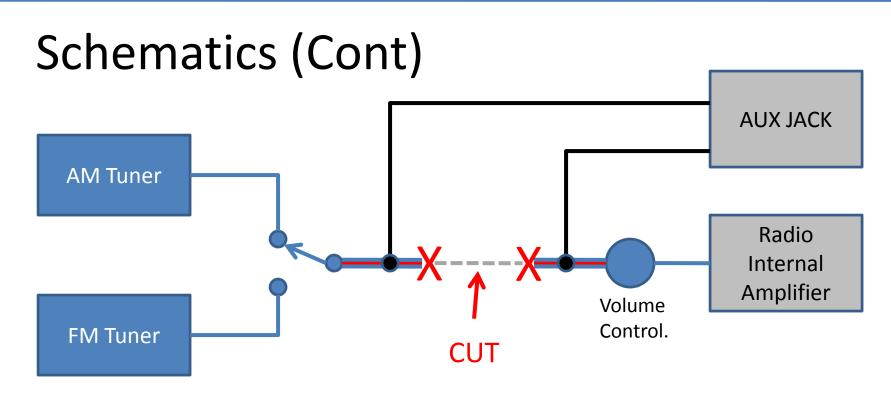
This is a description of what we will be doing inside the radio. Basically you can see here a simplified block diagram of the radio. The AM Section or FM section is selected by the AM/FM switch and sent by the "Blue/RED" wire to the Volume control. The volume control then feeds the Amplifier section.
