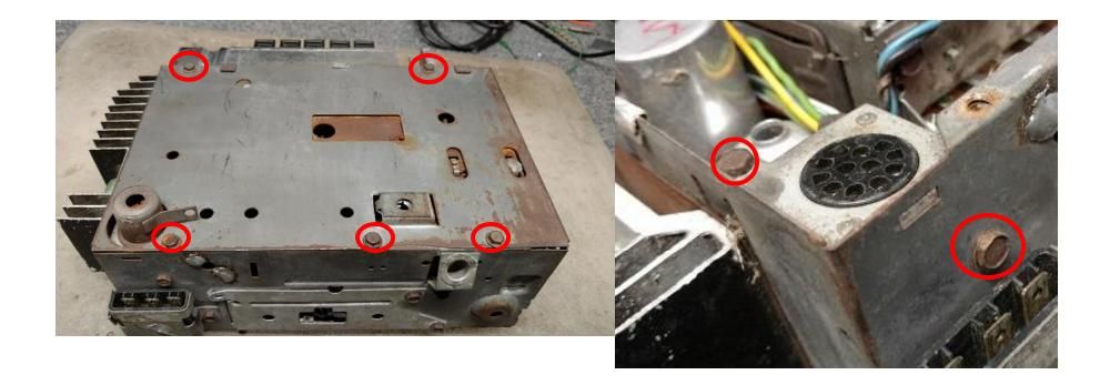
On the bottom of the radio, remove the shorting plug by pulling out on it. remove the 5 screws holding the bottom cover on and remove the bottom cover
