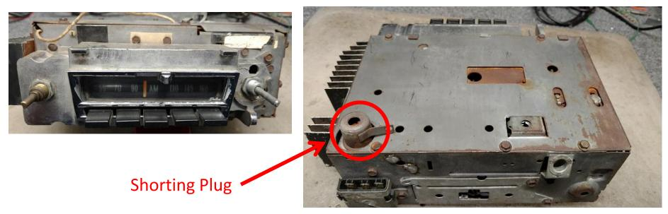
This instruction will show you how to connect an AUX input jack to the Late Model Corvair AM/FM radio with shorting plug in place ONLY. If you are using a multiplex unit with your radio, the AUX input should be added to the multiplex unit to allow stereo input. Use these instructions at your own risk- JCCRC is not responsible for any damage you do to your radio, car, self, family, pets, home or planet while using these instructions.
