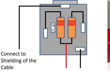
Here is the connection of the resistors and cable to the headphone jack.
