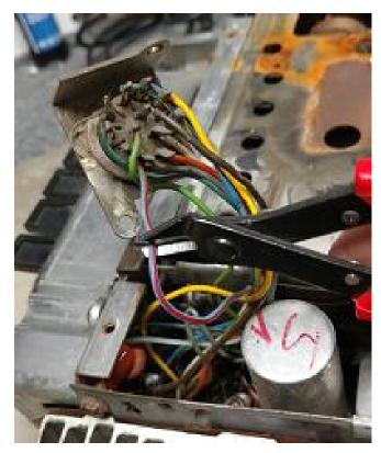
Lift out the socket to gain access to the wires. Locate the Blue wire with a red stripe.
