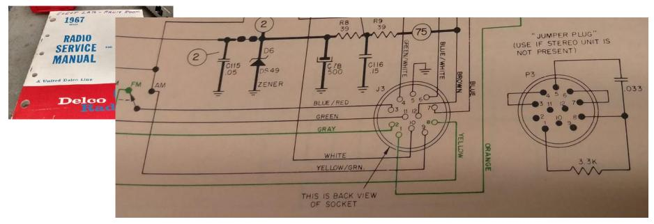
Pulling the schematic from the 1967 Delco radio manual (1965 is similar) we will focus on the Stereo plug. This picture shows the AM/FM switch on the far left. The switch takes Audio from the AM or FM section and sends it to the Audio section using the "BLUE/RED" wire connected to Pin #3 of the socket. This "Blue/Red" wire is where we will connect the AUX input.
