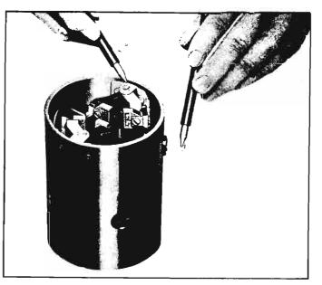
Fig. 8-46—Field Coil Test for Ground
