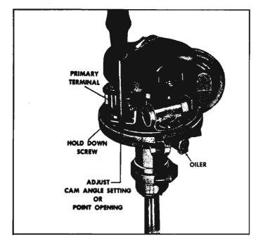
Fig. 8-55-Point Adjustment
