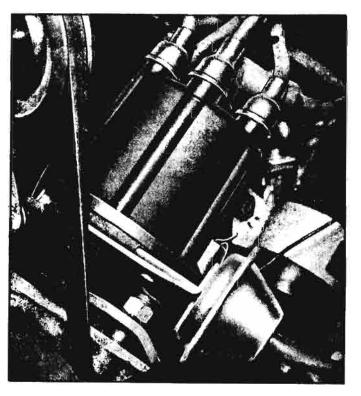
Fig. 8-60—Distributor Installed
