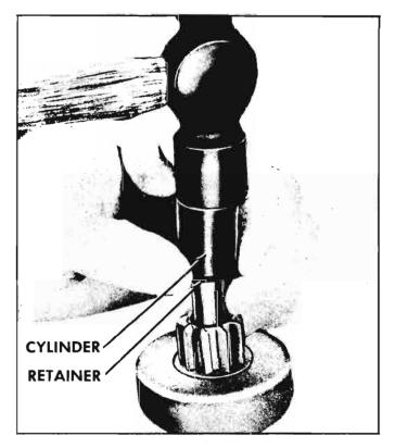
Fig. 8-42-Driving Retainer Off Snap Ring
