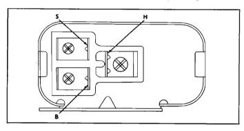
Fig. 8-120—Horn Relay Terminals
