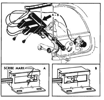
Fig. 8-110—Neutral Safety Switch Installation
