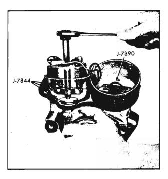
Fig. 8-152-Removing Field Coil with Tool J-7844
