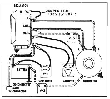
Fig. 8-5—Checking Generator Circuit Resistances
