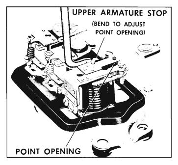
Fig. 8-33-Adjusting Cutout Relay Point Opening
