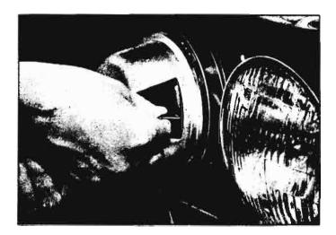
Fig. 8-103—Removing Aimer from Headlamp
