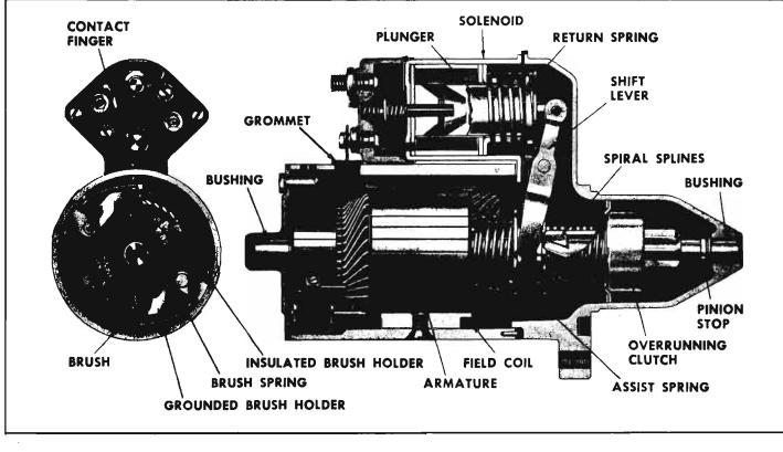
Fig. 8-38-Starting Motor Cross Section
