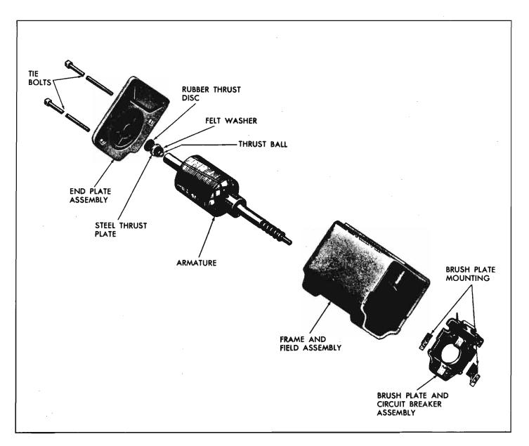
Fig. 8-129-Wiper Motor-Exploded View
