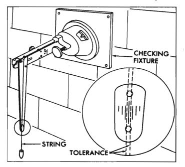
Fig. 8-96—Checking Horizontal Calibration
