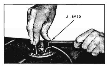
Fig. 8-118—Removing Fuel Tank Gauge Unit
