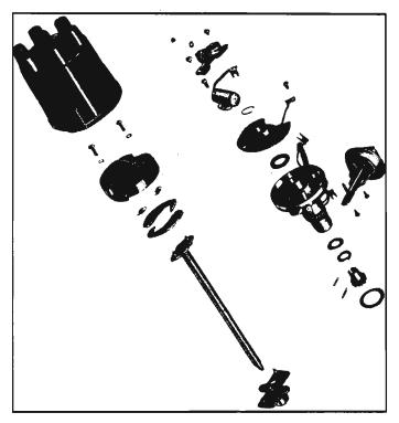
Fig. 8-59-Distributor Exploded View
