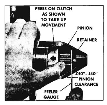
Fig. 8-50—Checking Pinion Clearance
