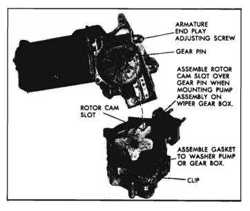
Fig. 8-132—Mounting Washer Pump to Gear Box
