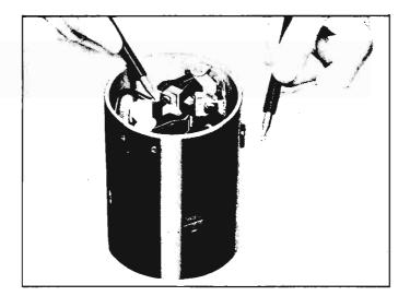
Fig. 8-45-Field Coil Test for Open Circuit
