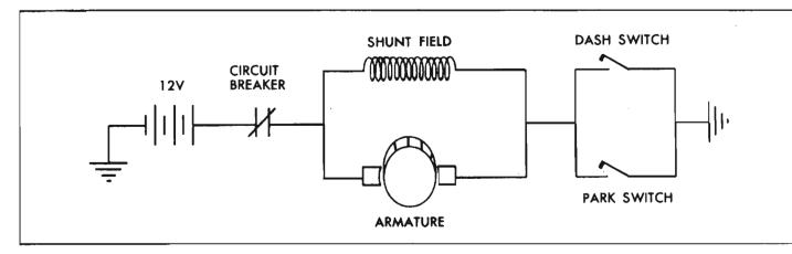
Fig. 8-125-Wiper Motor Circuit
