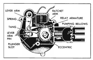
Fig. 8-136—Washer Pump Components
