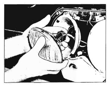
Fig. 8-91—Connecting Sealed Beam Unit
