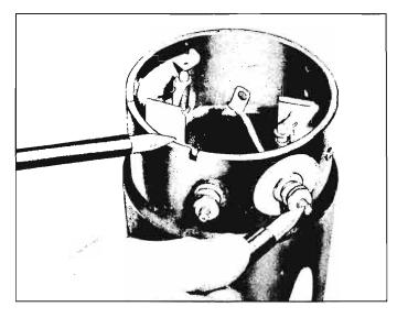
Fig. 8-24—Field Coil Test for Ground
