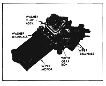
Fig. 8-124—Windshield Wiper and Washer Assembly
