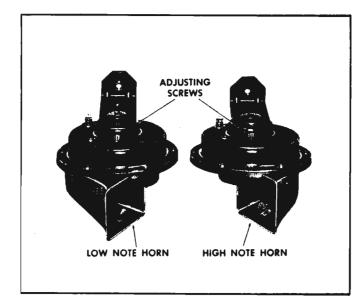
Fig. 8-121—Horn Adjustment
