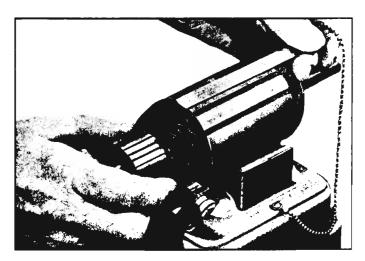
Fig. 8-20—Armature Test for Shorts
