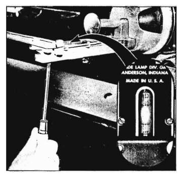
Fig. 8-99—Turning Level Adjusting Screw to Calibrate Aimer
