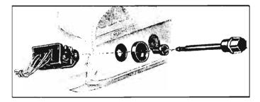
Fig. 8-106—Lighting Switch—Exploded View of Installation
