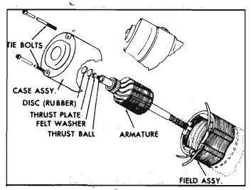
Fig. 8-150-Wiper Motor-Exploded View
