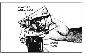
Fig. 8-130-Removing Gear Box
