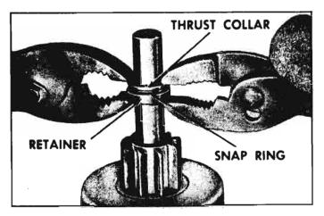
Fig. 8-48—Forcing Snap Ring Into Retainer
