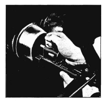
Fig. 8-97—Installing Aimer on Headlamp Unit
