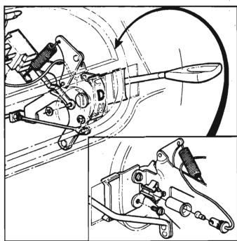
Fig. 5-161—Automatic Transmission Control Installation
