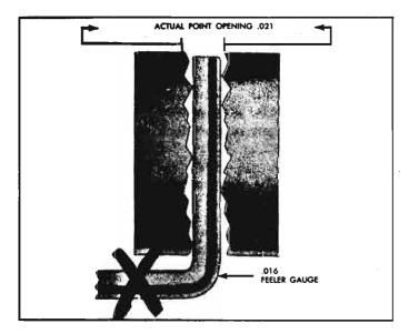
Fig. 8-54—Inaccurate Gauging of Rough Points
