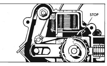
Fig. 8-137—Washer Pump Relay Energized
