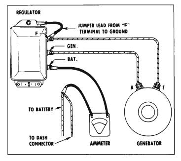
Fig. 8-12-Checking for Oxidized Contact Points
