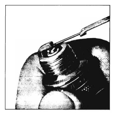
Fig. 8-64—Setting Spark Plug Gap
