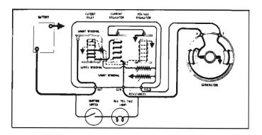
Fig. 8-2-Generating Circuit
