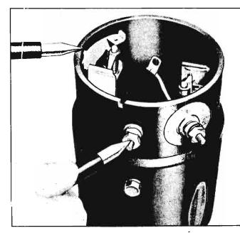
Fig. 8-25—Positive Terminal Test for Ground
