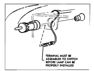
Fig. 8-112-instrument Panel Compartment Lamp Switch Installation
