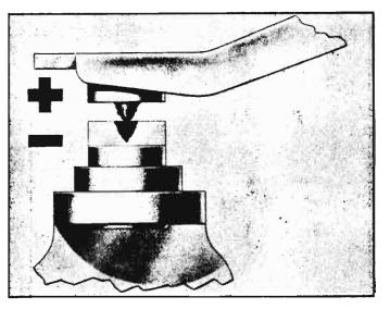
Fig. 8-52—Material Transfer—Negative to Positive Point
