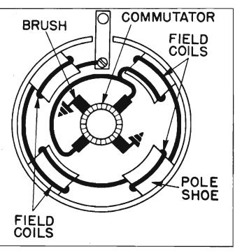
Fig. 8-35-Starting Motor Circuit-Series Field Colls
