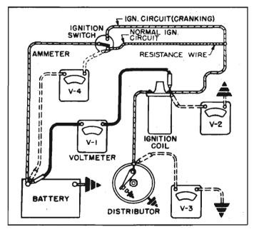
Fig. 8-51—Ignition Circuit Checks
