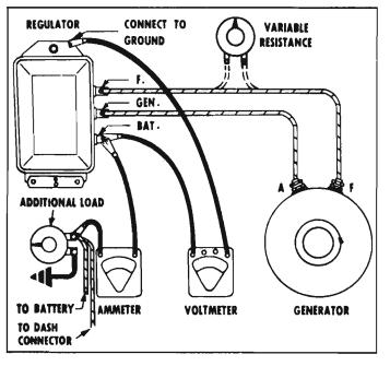
Fig. 8-11—Checking Current Regulator Setting
