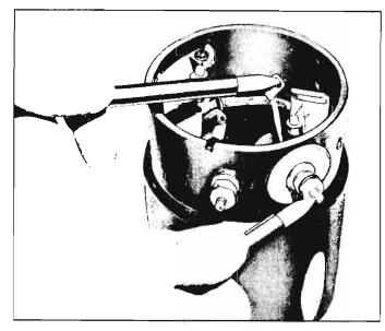
Fig. 8-23-Field Coil Test for Open Circuit
