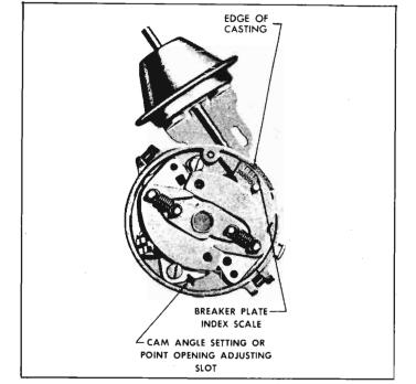
Fig. 8-57—Breaker Plate Positioning
