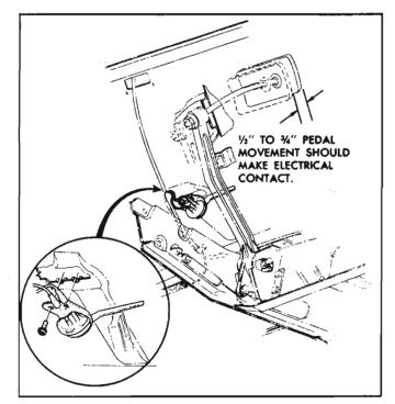
Fig. 8-158-Stoplight Switch Adjustment
