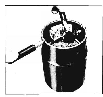
Fig. 8-26-Positive Brush Test for Ground
