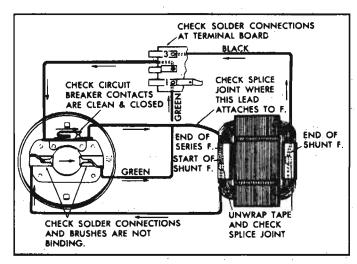
Fig. 8-151-Shunt Field Circuit
