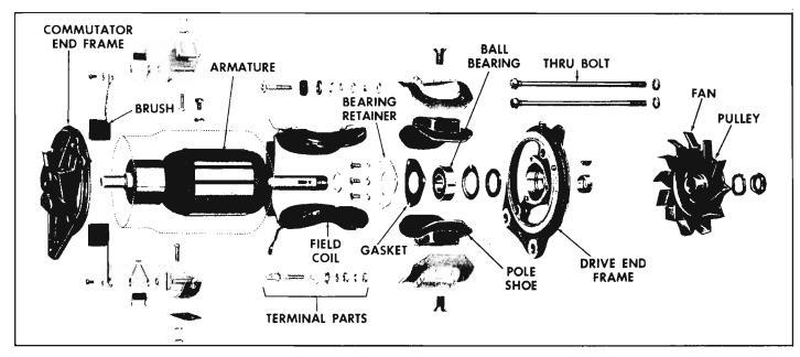
Fig. 8-17—Generator—Exploded View
