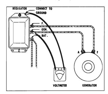
Fig. 8-10-Checking Cutout Relay Closing Voltage
