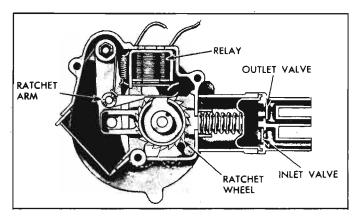
Fig. 8-138—Washer Pump Discharge Stroke
