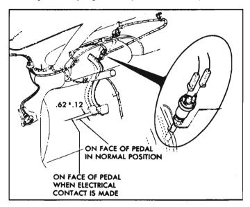
Fig. 8-107—Stoplight Switch Installation
