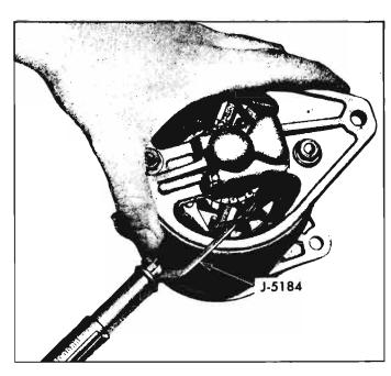
Fig. 8-19-Checking Brush Spring Tension
