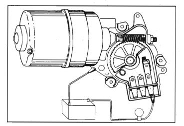
Fig. 8-154—Test Lamp Connections
