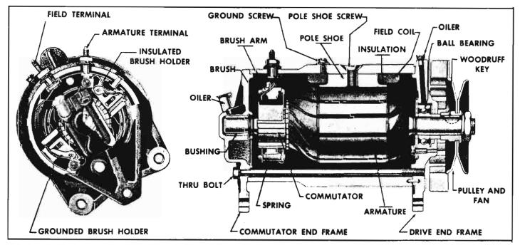
Fig. 8-4-Generator Cross-Section
