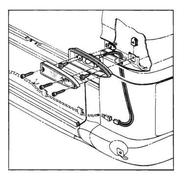
Fig. 8-159—Tail Lamp Assembly
