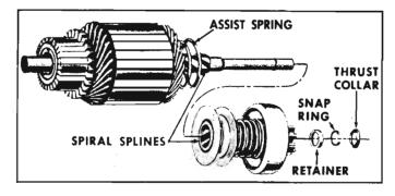
Fig. 8-41—Exploded View of Armature and Overrunning Clutch Assembly
