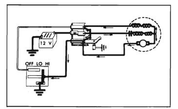
Fig. 8-145-"Hi" Speed Circuit
