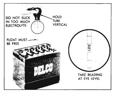
Fig. 8-13-Testing Specific Gravity of Battery (Typical)
