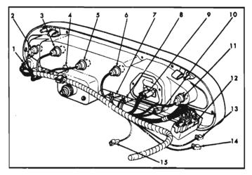
Fig. 8-160—Instrument Cluster Wiring
