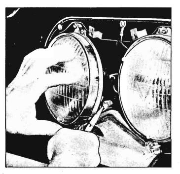
Fig. 8-88—Removing Retaining Ring Spring
