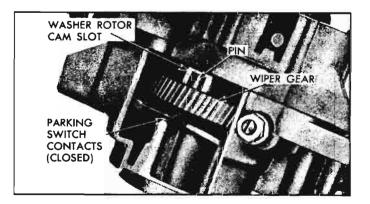
Fig. 8-126-Parking Switch Contacts in Operating Position
