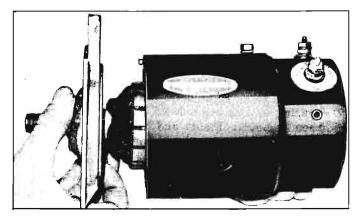
Fig. 8-15—Removing End Frame and Armature from Generator
