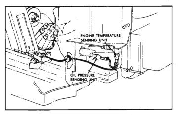
Fig. 8-117—Oil Pressure and Cylinder Head Temperature Senders
