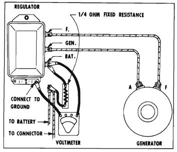
Fig. 8-6—Checking Voltage Regulator Setting
