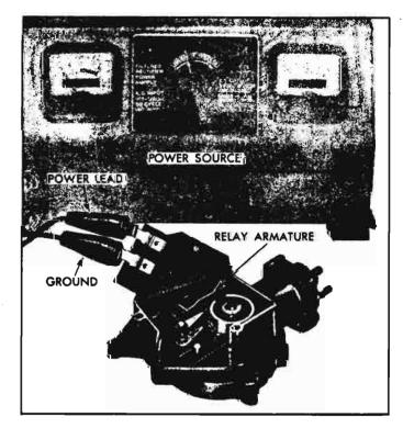
Fig. 8-143—Checking Detached Washer Pump
