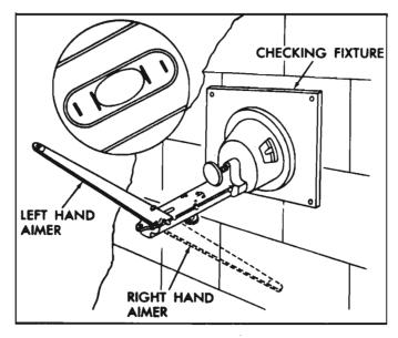
Fig. 8-95-Checking Vertical Calibration
