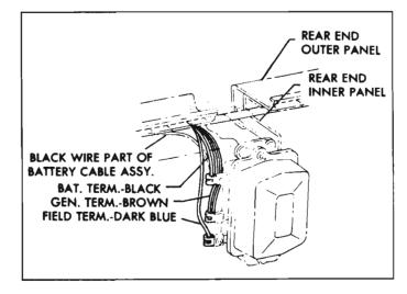
Fig. 8-29-Regulator Installed
