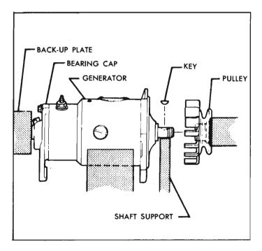
Fig. 8-27—Pulley Assembly
