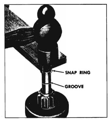
Fig. 8-47—Forcing Snap Ring Over Shaft
