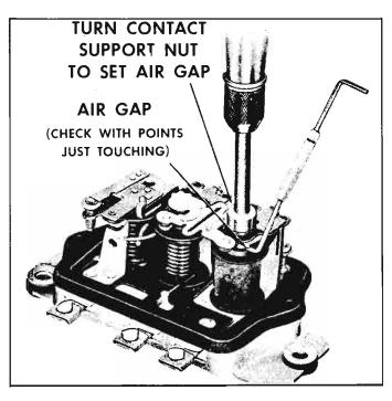
Fig. 8-34—Adjusting Regulator Air Gap
