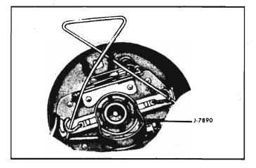
Fig. 8-149—Retaining Armature Brushes
