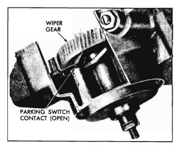
Fig. 8-127—Parking Switch Contacts in Park Position
