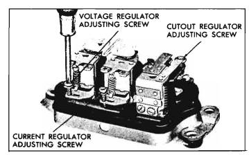
Fig. 8-7—Regulator Adjusting Screws
