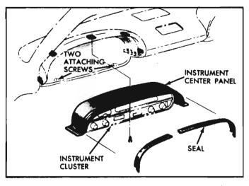
Fig. 8-116—Instrument Cluster Attaching Screws
