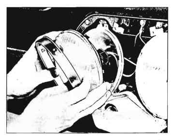
Fig. 8-90-Removing Retaining Ring, Sealed Beam Unit and Mounting Ring
