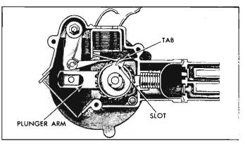
Fig. 8-141-Washer Pump Idling
