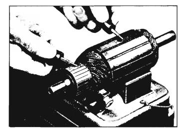
Fig. 8-21—Armature Test for Ground
