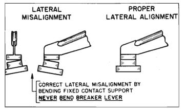
Fig. 8-56—Alignment of Points
