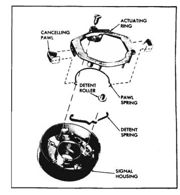
Fig. 8-122—Exploded View—Direction Signal Mechanism
