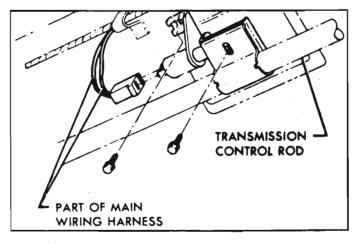
Fig. 8-111-Back-Up Lamp Switch Installation
