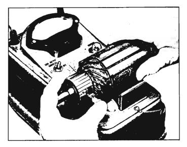
Fig. 8-22—Armature Test for Open Circuit
