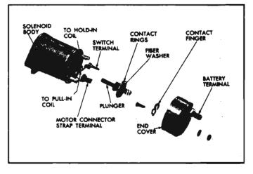
Fig. 8-49—Exploded View of Solenoid
