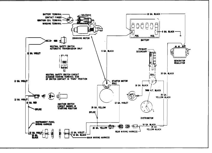
Fig. 8-155—ignition Starting Energized
