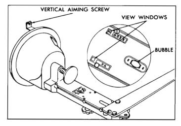
Fig. 8-98—Selecting Level Aiming Area
