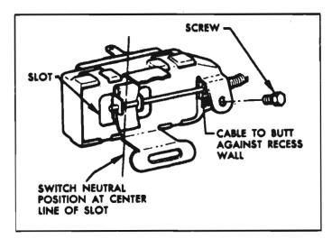
Fig. 8-123—Direction Signal Switch
