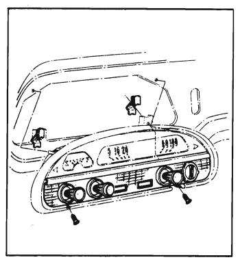
Fig. 8-162-Instrument Panel Removal
