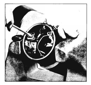
Fig. 8-16-Removing Brush Leads
