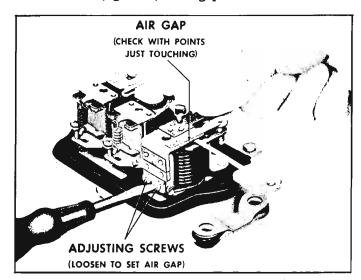
Fig. 8-32—Adjusting Cutout Relay Air Gap
