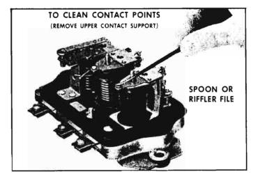
Fig. 8-30—Cleaning Regulator Contact Points
