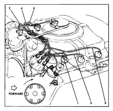
Fig. 8-61—Distributor, Spark Plug Wire and Cylinder Numbering
