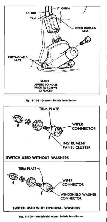
assembly and loosely install the two attaching screws.
