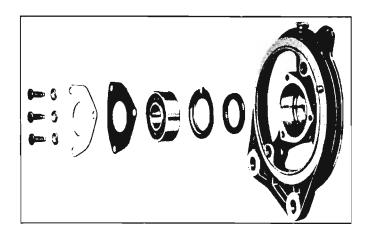
Fig. 8-18—Exploded View of Drive End Frame Assembly
