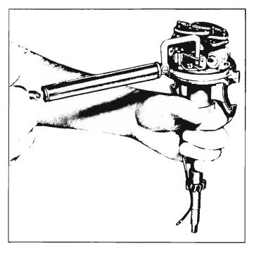
Fig. 8-58—Checking Breaker Arm Spring Tension
