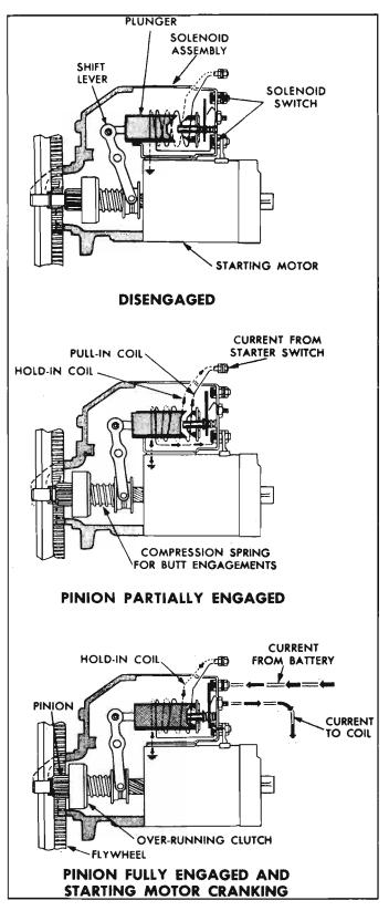
Fig. 8-37—Solenoid Operation
