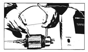
Fig. 8-44—Armature Test for Ground
