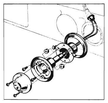
Fig. 8-113—Tail, Stop and Back-Up Lamp—Expleded View of Installation (Typical)
