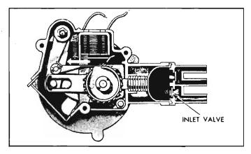
Fig. 8-139-Washer Pump Inlet Stroke
