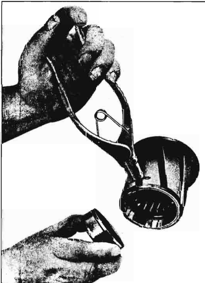
Fig. 6D-15—Removing Synchronizer Ring with J-932
