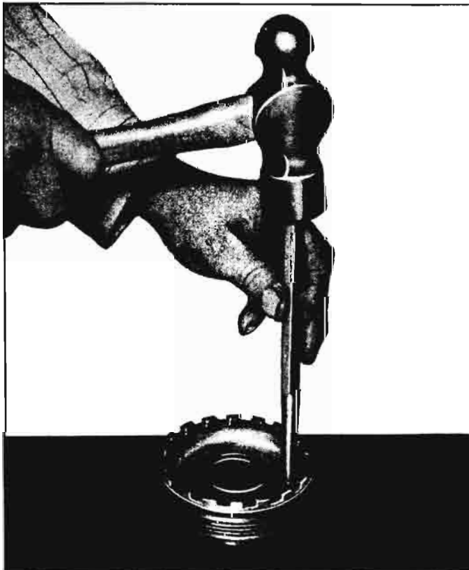
Fig. 6C-28—Sealing Drilled Holes in Adjusting Sleeve with Lead Balls
