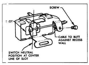
Fig. 4-42—Installation of Cable in Switch
