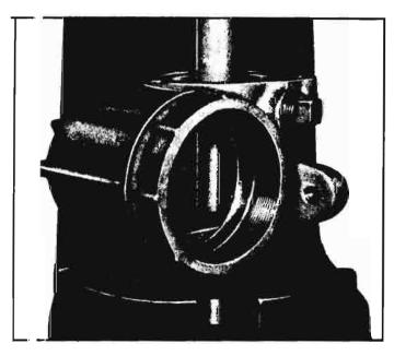
Fig. 4-14—Removing Sector Shaft Bushing
