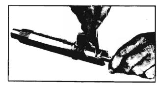
Fig. 4-51—Checking Lash Adjuster End Clearance
