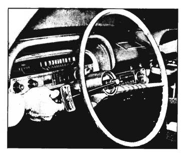
Fig. 4-6—Checking Steering Wheel Turning Torque
