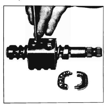
Fig. 4-16—Placing Balls in Nut
