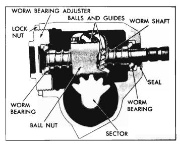
Fig. 4-1-Steering Gear Worm and Ball Nut Circuits
