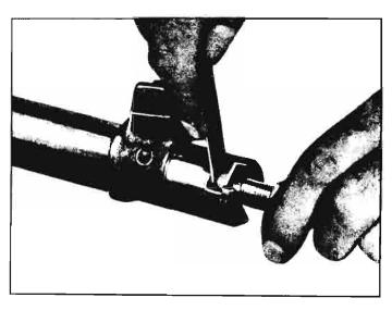
Fig. 4-19—Checking Lash Adjuster End Clearance
