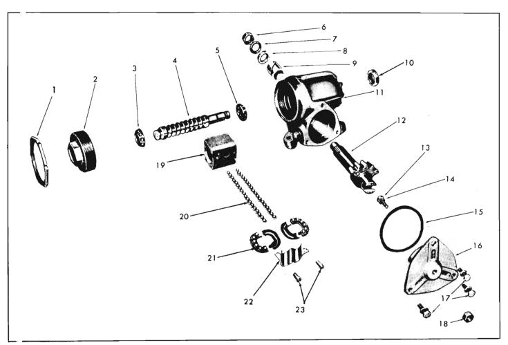
Fig. 4-11—Exploded View of Steering Gear
