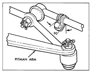
Fig. 4-28—Clamp Flange Position
