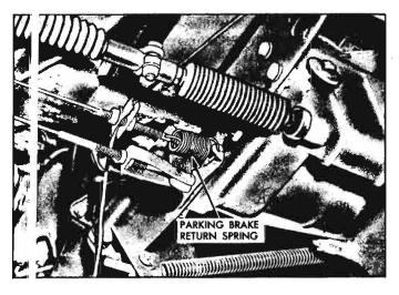
Fig. 4-25—Parking Brake Return Spring
