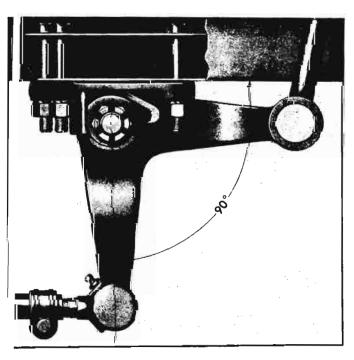
Fig. 4-37—Angle of Relay Arm to Frame
