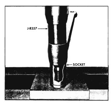
Fig. 4-30—Installing Bushing
