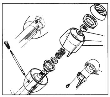
Fig. 4-39-Exploded View of Steering Wheel
