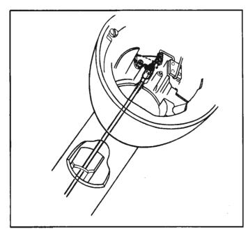
Fig. 4-40—Pivoting Cable Clamp to Install Housing
