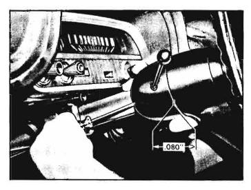
Fig. 4-7—Adjusting Turn Signal Housing Clearance
