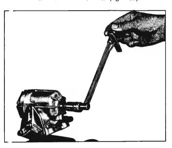
fig. 4-20-Checking Worm Bearing Pre-Load
