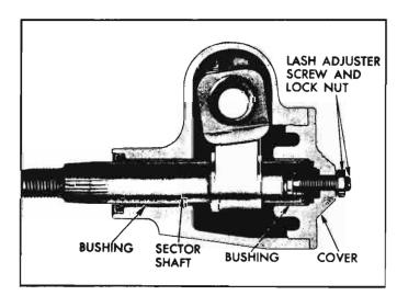
Fig. 4-4—Sector Gear and Pitman Shaft
