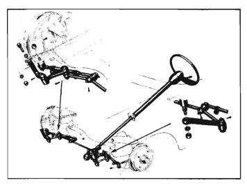
Fig. 4-2—Steering Linkage
