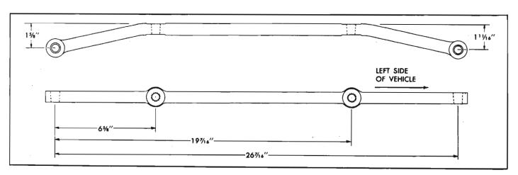
Fig. 4-55—Relay Rod
