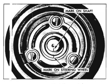
Fig. 4-9—Steering Wheel Alignment Marks
