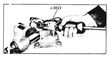
Fig. 4-48—Removing Bearing Cup
