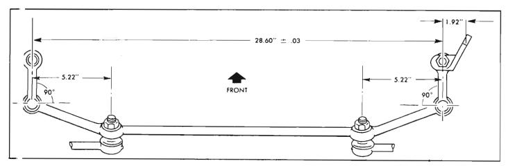
Fig. 4-31—Steering Linkage Alignment
