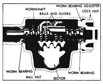
Fig. 4-44—Cross-Section of Steering Gear
