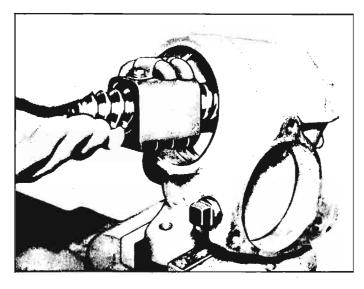
Fig. 4-13—Removing Wormshaft and Ball Nut
