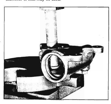
Fig. 4-47—Pressing Bushing with J-1614
