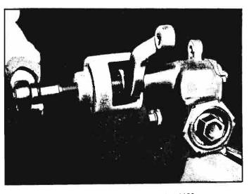
Fig. 4-45—Pulling Pitman Arm with J-6632
