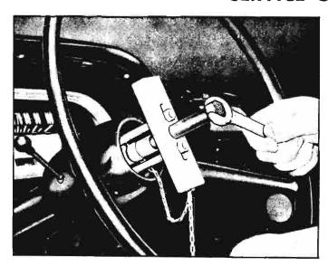
Fig. 4-8—Steering Wheel Removal
