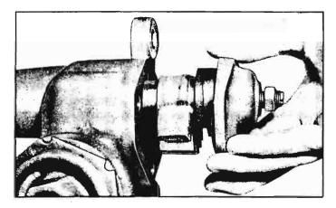
Fig. 4-46—Removing Cover and Sector Shaft
