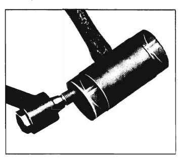
Fig. 4-29—Removing Pivot Bolt
