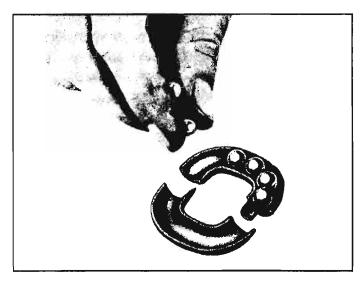
Fig. 4-17—Filling Ball Guides
