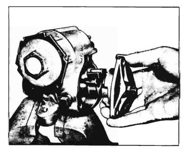
fig. 4-12—Removing Pitman Shaft
