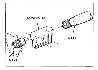
Fig. 4-22—Alignment of Steering Gear Shaft, Steering Shaft and Coupling
