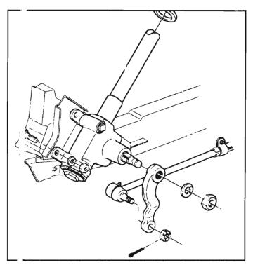
Fig. 4-52—Installation of Steering Gear
