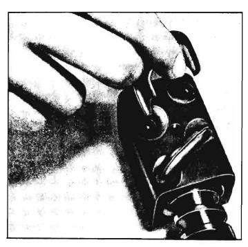
Fig. 4-18—Inserting Ball Guides in Nut
