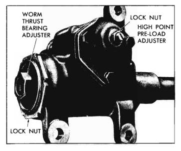
Fig. 4-34—Steering Gear Adjustment Points
