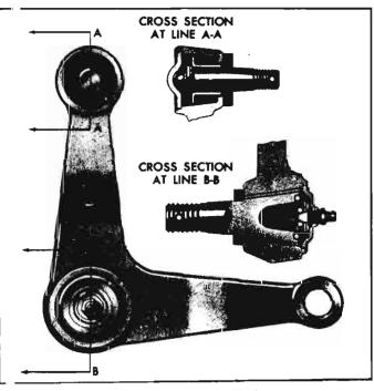
Fig. 4-53—Relay Arm Assembly
