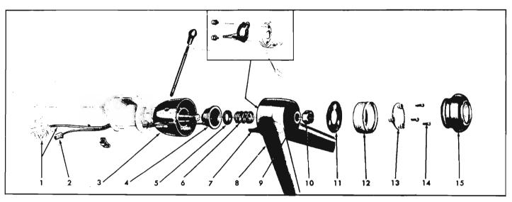
Fig. 4-24—Exploded View of Upper Mast Jacket and Steering Wheel
