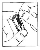
Fig. 1-16—Inserting tumbler springs.
