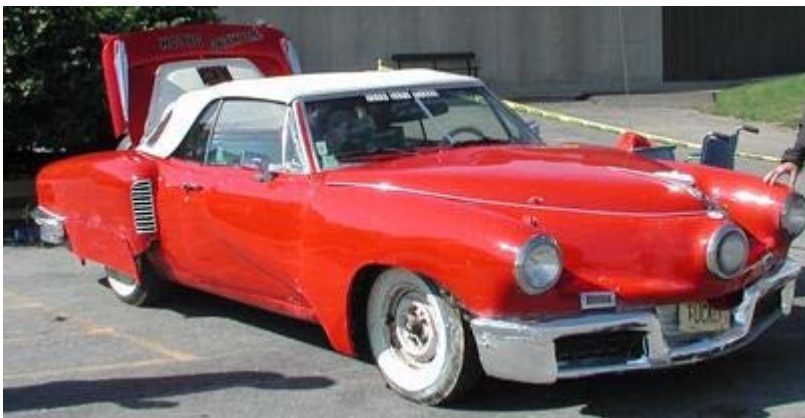
Tucker replica built on a Corvair frame
