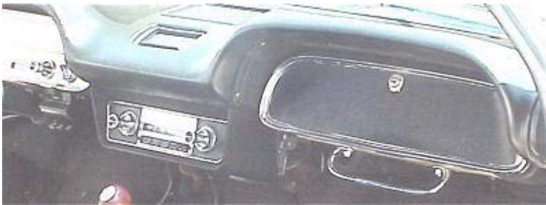
Dark vinyl covering on radio faceplate and glovebox door with Grab-rail option.
