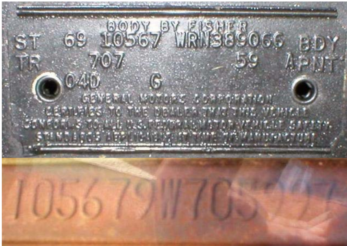
Fisher bodytag from # 5997 on top, Vin tag from dash on bottom
