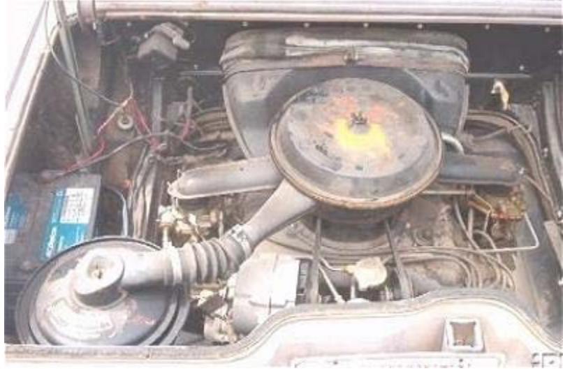
Late model Desert air package. Notice plenum
