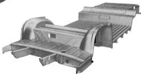
Heavily ribbed and contoured Greenbrier floor panel assembly.
