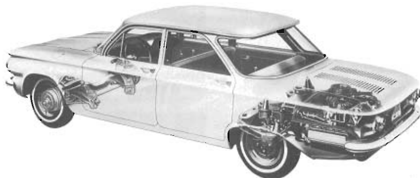
Corvair Quadri-Flex 4-wheel independent suspension and transaxle-drive rear-mounted Unipack Power Team.
