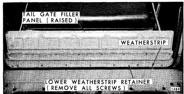
Fig. 9-49—Tail Gate Weatherstrip Retention
