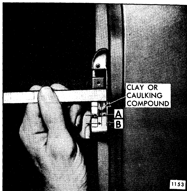
Fig. 9-46—Tail Gate Lock Striker Caulking Check
