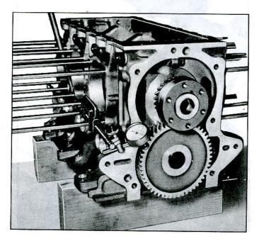
Fig. 62-Measuring Timing Gear Backlash
