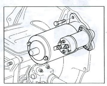
Fig. 2s-Starting Motor Installed
