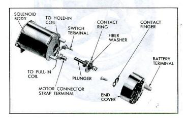
Fig. 12s-Exploded View of Solenoid
