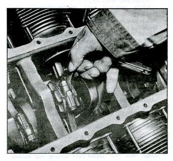
Fig. 65-Connecting Rod Side Clearance
