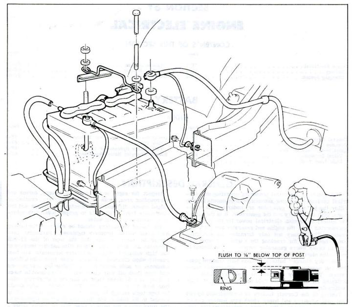
Fig. 1b-Battery Installation
