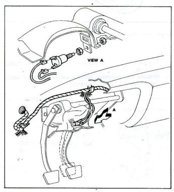
Fig. 13-Stoplight Switch Installation
