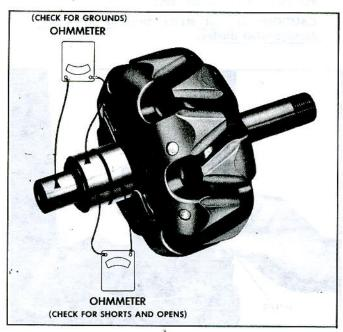
Fig. 16c-Checking Rofor for Grounds or Opens
