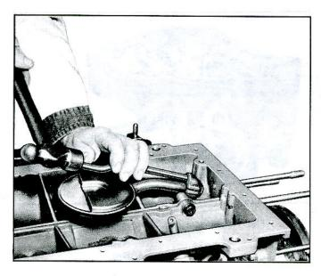
Fig. 108-Installing Pick-Up Screen and Tube
