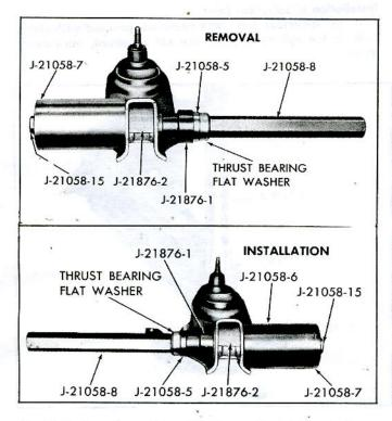
Fig. 3-20-Removing and Installing Lower Control Arm Bushings
