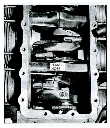
Fig. 39-Connecting Rod Bearing Replacement
