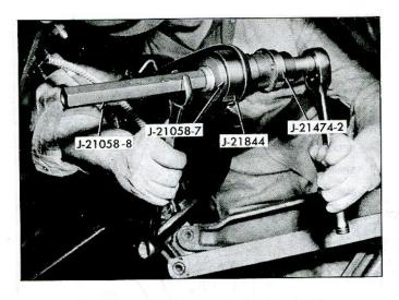
Fig. 81-Installing Torque Control Arm Bushing
