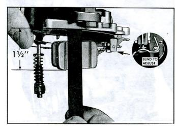
Fig. 12-Measuring Float Drop
