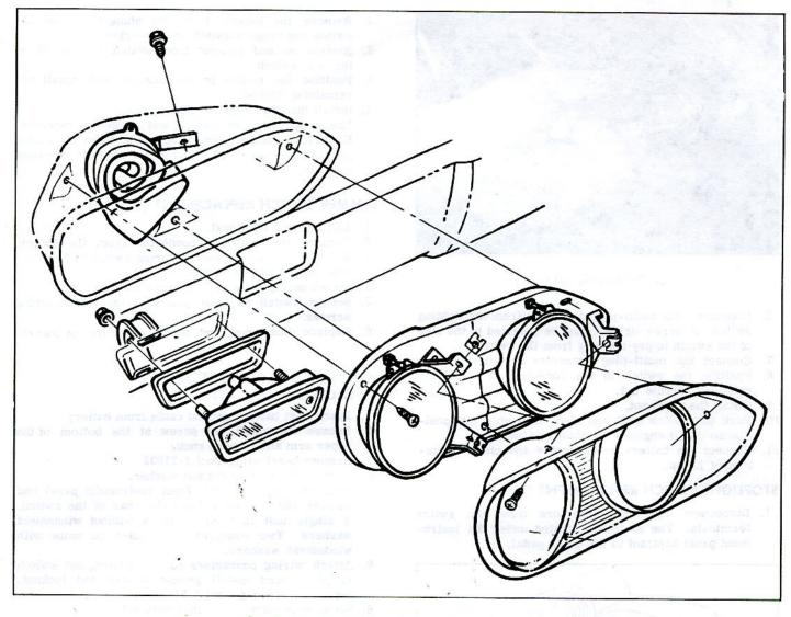
Fig. 9—Headlamp, Parking Lamp and Horn Assemblies
