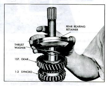
Fig. 7B–14—Installing 1–2 Synchronizer, First Gear, and Rear Bearing Retainer on Mainshaft
