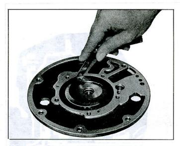
Fig. 7E-31-Checking Driven Gear-to-Pump Body Clearance
