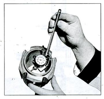
Fig. 100-Measuring Cylinder Bore
