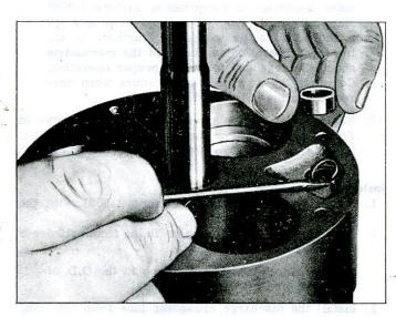
Fig. 55—Installing Discharge Crossover Tube
