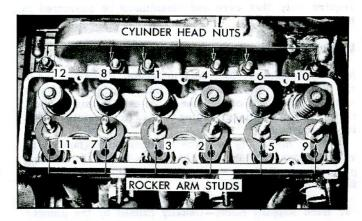
Fig. 34-Cylinder Head Torque Sequence
