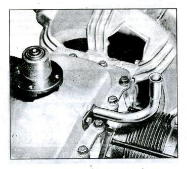
Fig. 67-Crankcase Vent Tube
