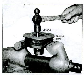
Fig. 7E-46-Removing Short Planet Pinion
