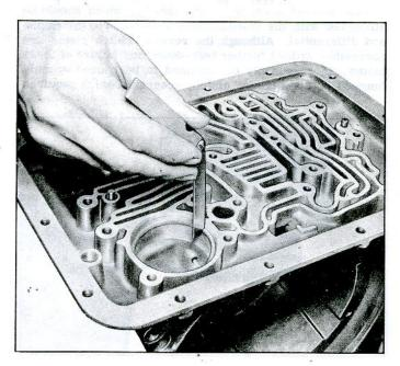
Fig. 7E-12-Measuring Low Servo Piston Ring Gap
