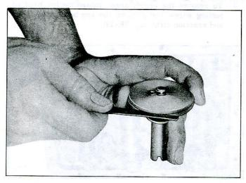
Fig. 7E-13-Measuring Piston-to-Ring Clearance
