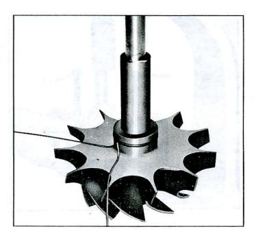
Fig. 49-Ring Compressed Using Tag Wire
