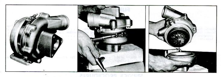
Fig. 55—Removal of the Turbine Housing for Installation of Replacement Turbocharger
