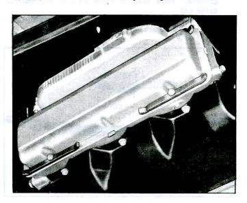
Fig. 36-Rocker Arm Cover Installed
