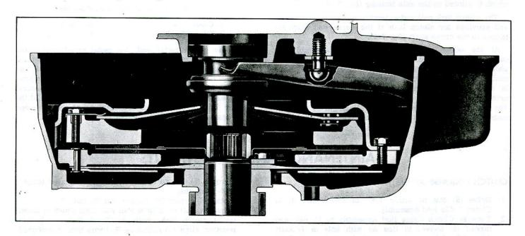
Fig. 7-1-Clutch Cross-Section
