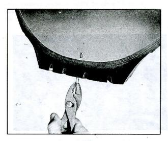
Fig. 12—Installing Filler Rubber in Hole
