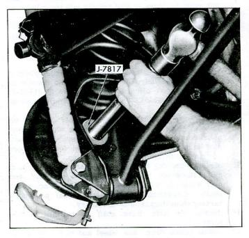
Fig. 71—Installing Spindle Support Inner Bearing
