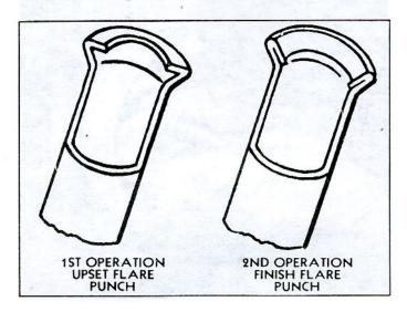
Fig. 12-Flaring Operation-First and Second Flare
