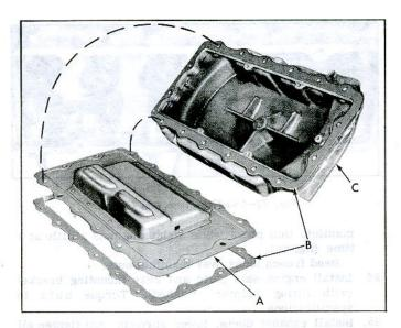
Fig. 66-Crankcase Cover and Vent
