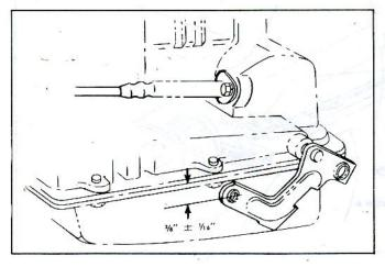
Fig. 7E-7-Cable Installation Check Diagram
