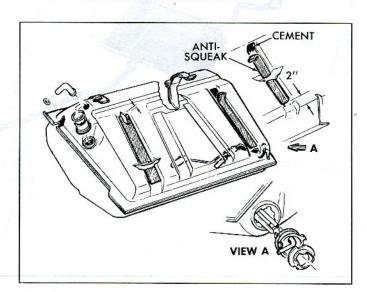
Fig. 3-Fuel Tank and Metering Unit
