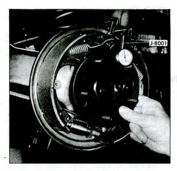
Fig. 63-Measuring Wheel Bearing End Play
