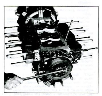
Fig. 52-Cylinder Holding Fixture
