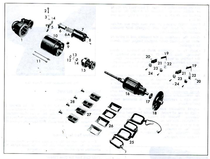
Fig. 3s-Starting Motor Parts Layout
