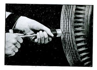
Fig. 8-Filling Hole with Sealing Gun
