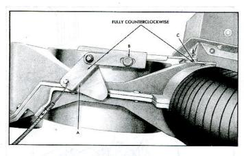
Fig. 8-"Heat" Control Cable
