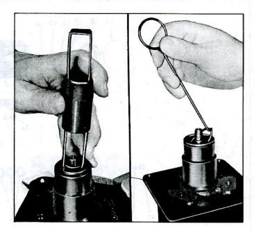
Fig. 41-Removing Seal Seat and "O" Ring
