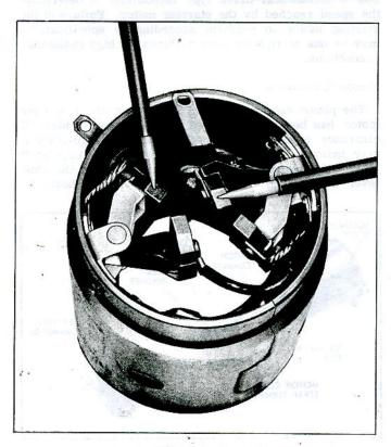
Fig. 8s-Field Coil Ground Test
