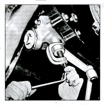
Fig. 3-Removing Pitman Arm With Tool J-6627
