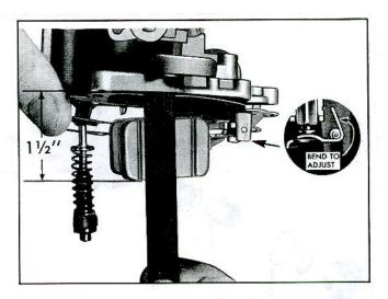
Fig. 23-Measuring Float Drop
