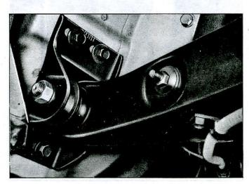
Fig. 62-Toe-in Adjusting Bracket Location
