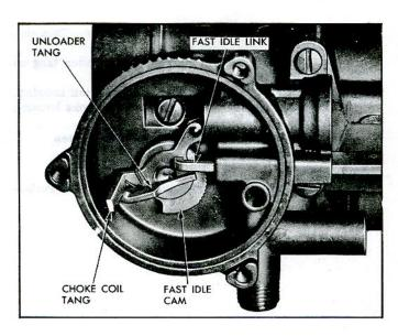
Fig. 34—Choke Housing and Fast Idle Linkage
