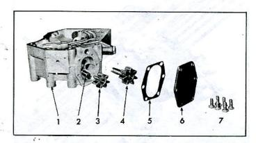
Fig. 112-Oil Pump-Exploded View
