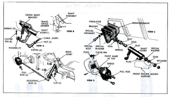
Fig. 7-9-Clutch Linkage Exploded
