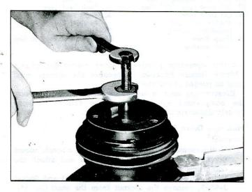
Fig. 32—Removing Hub and Drive Plate Assembly
