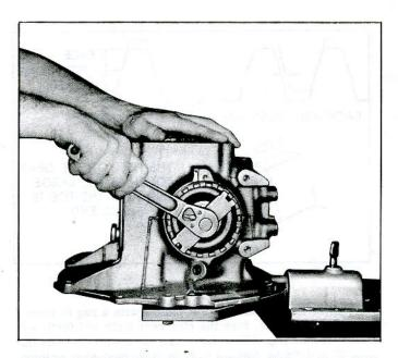
Fig. 46-Tightening Side Bearing Adjusting Sleeve with J-8342
