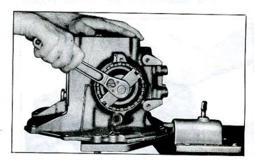
Fig. 14—Removing Side Bearing Adjusting Sleeve with J-8342
