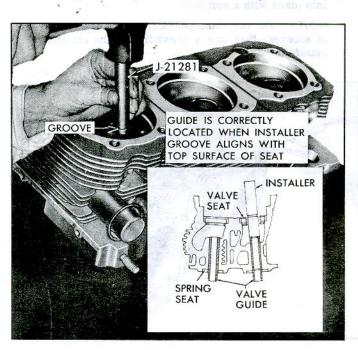
Fig. 90—Installing Valve Guide
