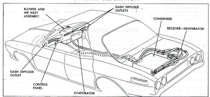
Fig. 9-Corvair All-Weather Air Conditioning System
