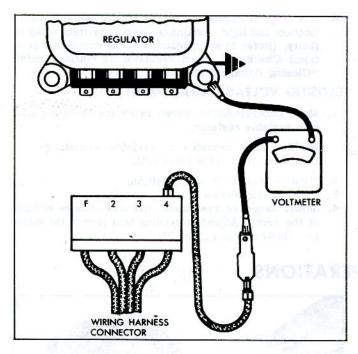
Fig. 9c-Circuit Resistance Wire Test
