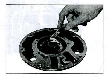
Fig. 7E-32—Checking Driven Gear-to-Crescent Clearance
