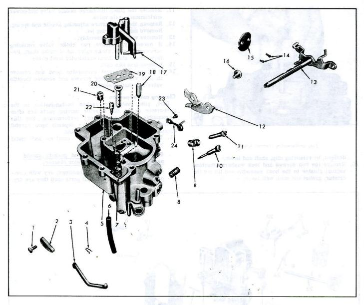
Fig. 8-Carburetor Body-Exploded View
