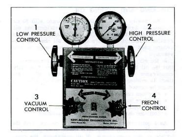
Fig. 22-Charging Station Controls
