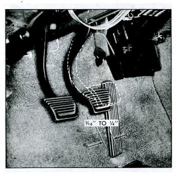
Fig. 6-Brake Pedal Free Movement
