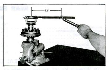
Fig. 59-Checking Clutch Pack Preload-On the Bench
