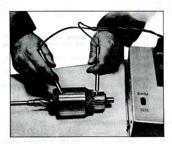
Fig. 6s-Armature Ground Test
