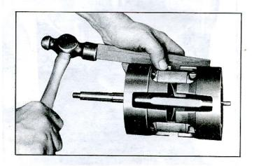
Fig. 48-Separating Cylinder Halves
