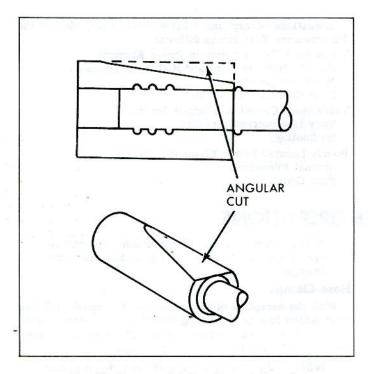
Fig. 21—Recommended Hose Removal Procedure
