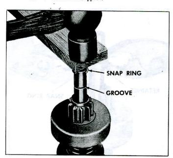
Fig. 9s—Forcing Snap Ring over Shaft
