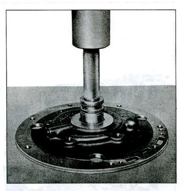
Fig. 7E-34-Installing Front Pump Bushing with J-8360-5
