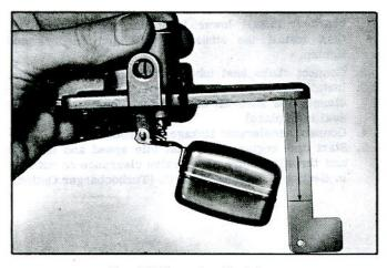
Fig. 32-Measuring Float Drop
