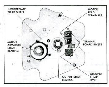
Fig. 32-Terminal Board-Single Speed Wiper
