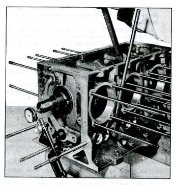
Fig. 60-Measuring Crankshaft End Play
