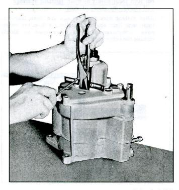
Fig. 7A-6—Locking Clutch Gear Retainer Expanded with J-8361
