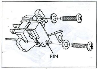
Fig. 21c-Brush Assembly-5.5" Delcotron
