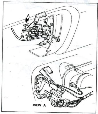
Fig. 16-Neutral Safety Switch Installation
