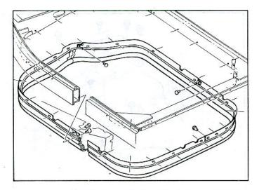
Fig. 20-Engine Seal and Retainer
