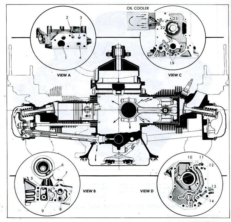
Fig. 19-Engine Lubrication
