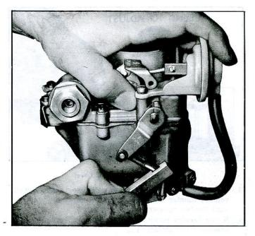
Fig. 13-Adjusting Pump Rod
