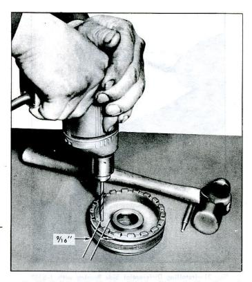
Fig. 25-Drilling Side Bearing Adjusting Sleeve for Race Removal
