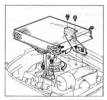
Fig. 57-Condenser Removal
