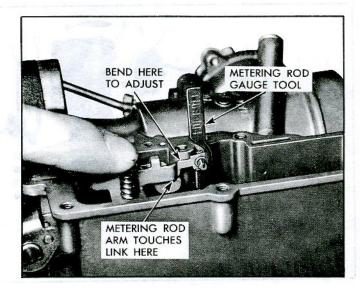
Fig. 30-Adjust Metering Rod Arm
