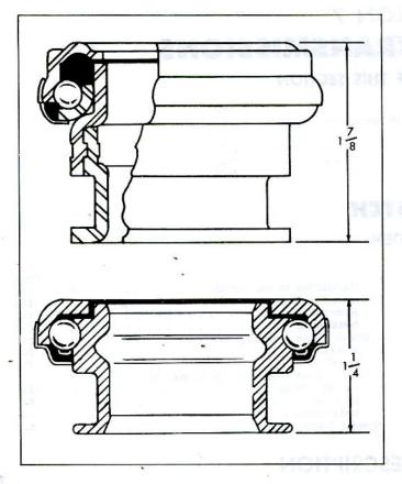
Fig. 7-2-Release Bearing Comparison
