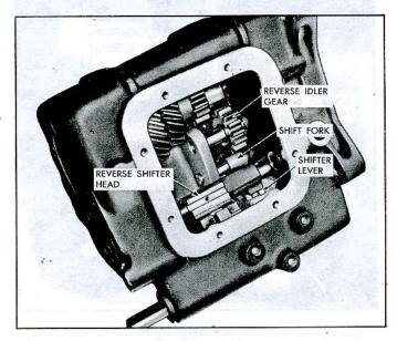
Fig. 7B-20-Reverse Shifter Head Installation
