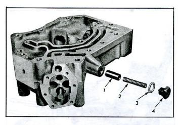
Fig. 113-Pressure Regulator-Exploded View
