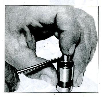
Fig. 94—Removing Ball Check Valve
