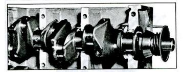
Fig. 56-Crankshaft Installed
