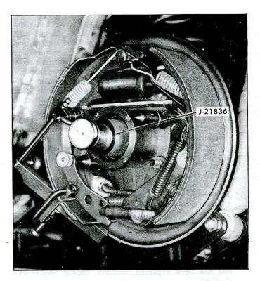
Fig. 73-Gauging Wheel Bearing Shim Requirement
