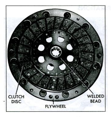
Fig. 7-7—Clutch Disc Installed
