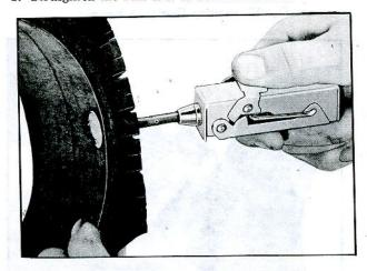
Fig. 21-Seating Plug to Complete Repair
