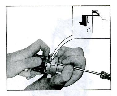
Fig. 9i-Unlocking Ignition Switch Connector
