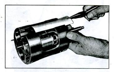
Fig. 46-Removing Suction Crossover Cover
