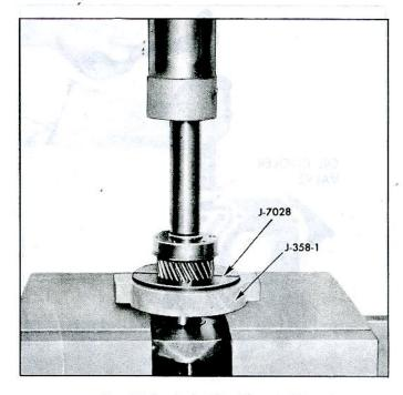
Fig. 120—Removing Crankshaft Gear
