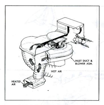
Fig. 2—Heater Inlet Duct and Blower Assembly
