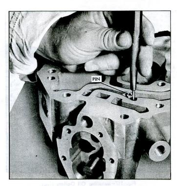
Fig. 116-Installing Pressure Regulator Groove Pin
