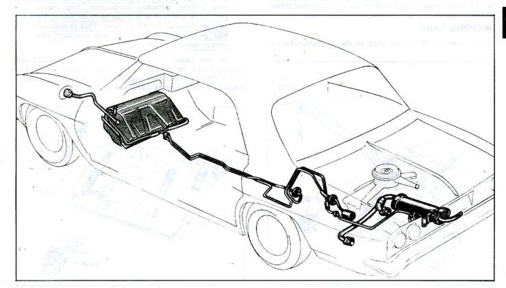
Fig. 1-Fuel Tank and Exhaust System
