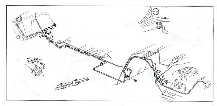
Fig. 4—Fuel Tank Lines (also by-pass for turbo-charged shown)
