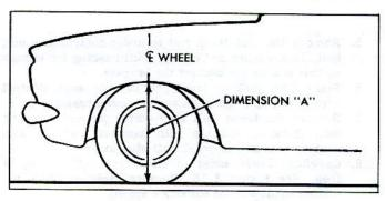
Fig. 3-14-Checking Riding Height
