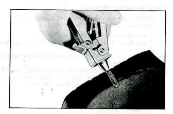
Fig. 18-Inserting Cement in Puncture
