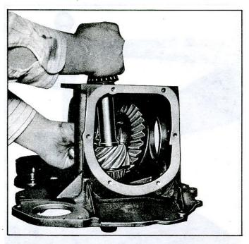
Fig. 45-Installing Pinion in Differential Carrier
