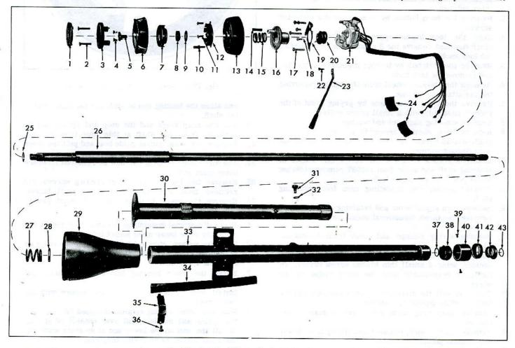
Fig. 19—Exploded View of Telescoping Mast Jacket
