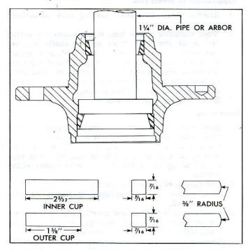
Fig. 3-7-Bearing Cup Removing Tools
