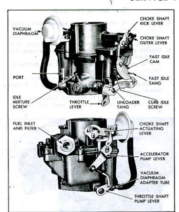
Fig. 1-Rochester HV Carburetor
