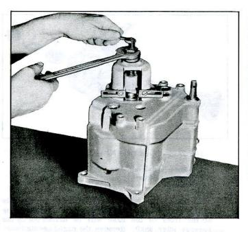
Fig. 7A-7-Pulling Clutch Gear and Bearing with J-8361
