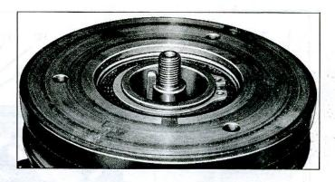
Fig. 33-Drive Plate Key Installed in Keywor
