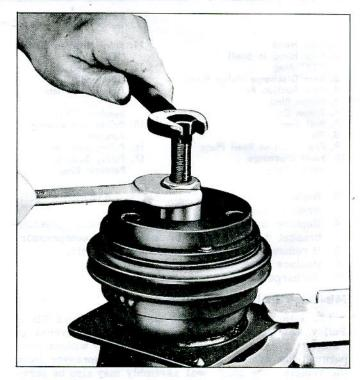
Fig. 34—Installing Hub and Drive Plate Assembly
