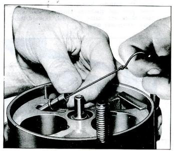
Fig. 45—Removing Oil Inlet Tube and "O" Ring
