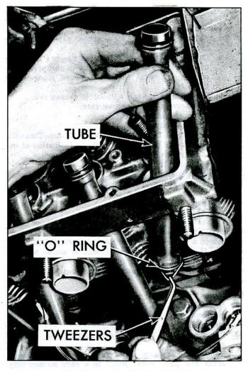
Fig. 33-Removing Push Rod Tubes
