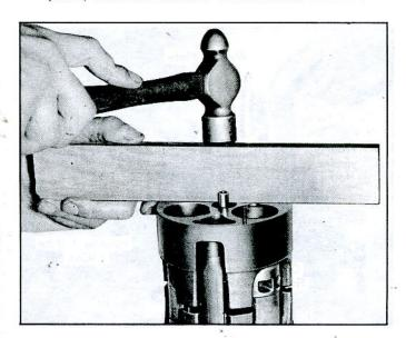
Fig. 51-Assembling Cylinder Halves
