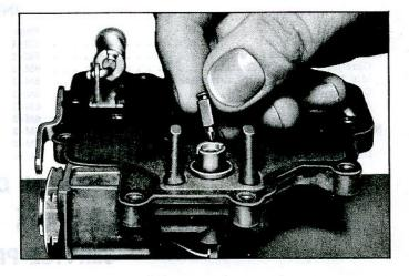
Fig. 4-Removing Float Needle
