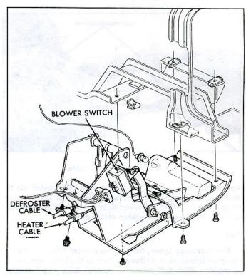
Fig. 7-Heater Control Panel Installation
