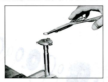
Fig. 7E-39—Installing Front Pump Shaft Thrust Washer Drive Hub Snap Ring
