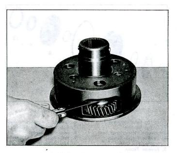
Fig. 7E-44-Checking Planet Gear End Clearance
