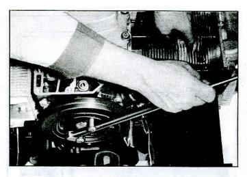
Fig. 76-Locating T.D.C. on Number Cylinder
