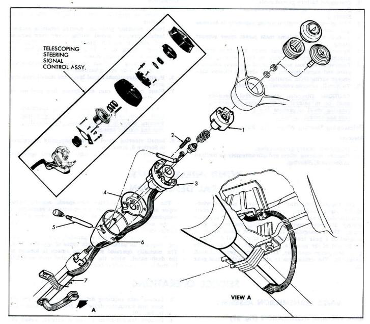
Fig. 28-Directional Signal Assemblies
