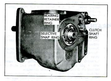
Fig. 7B-4-Clutch Gear and Bearing Snap Rings
