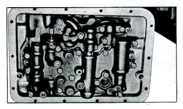
Fig. 7E-15-Valve Body Attaching Bolts
