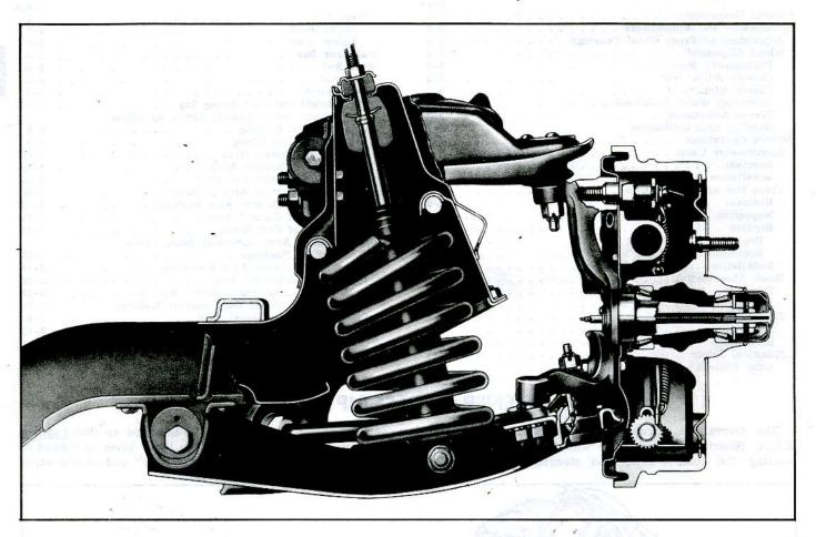
Fig. 3-2-Front Suspension Cross Section
