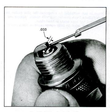
Fig. 11i—Setting Spark Plug Gap
