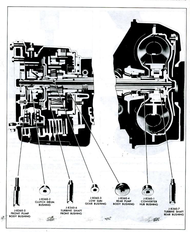
Fig. 7E-30—Powerglide Bushings and Installers
