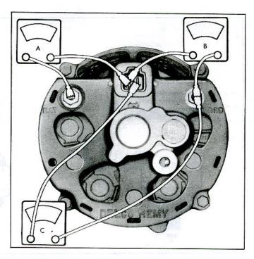
Fig. 7c-Delcotron Diode and Field Test
