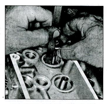
Fig. 93—Measuring Valve Spring Installed Height
