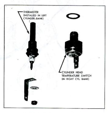
Fig. 41-Cylinder Head Temperature Sensing Units
