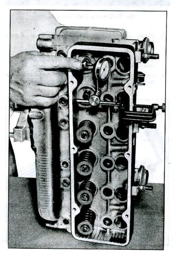
Fig. 82-Measuring Valve Stem Clearance
