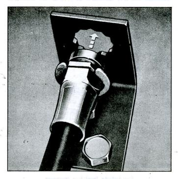
Fig. 7-Brake Line Support Bracket
