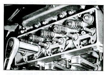
Fig. 32—Rocker Arm Studs and Push Rod Guides
