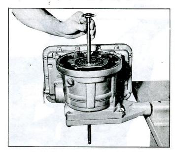
Fig. 7E-21—Removing Front Pump Drive Shaft
