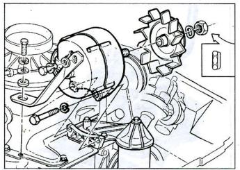
Fig. 13c-Delcotron Assembly
