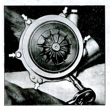
Fig. 36—Compressor Housing Retaining Bolts
