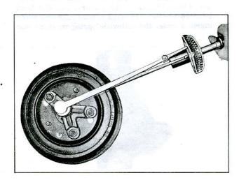
Fig. 53-Measuring Positraction Rotating Torque
