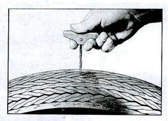
Fig. 15—Cleaning Puncture with Cleaning Needle been removed. Leave the needle in the puncture to prevent escape of air.
