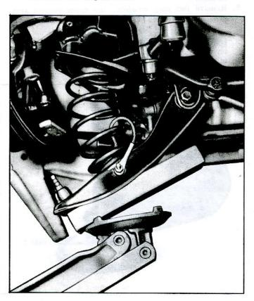
Fig. 3-21-Installing Coil Spring
