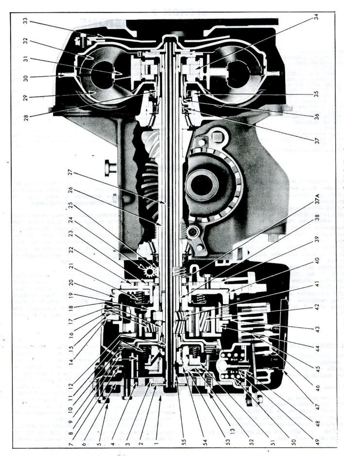
Fig. 7E-1-"Corvair" Powerglide-Cross Sectional View (L.D.F.C. Shown)
