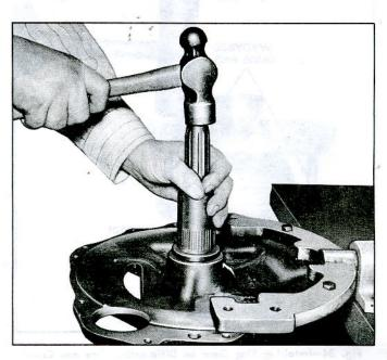
Fig. 38—Installing Converter Hub Seal with J-8340
