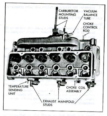
Fig. 91-Cylinder Head Assembly
