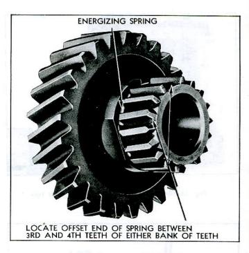
Fig. 7A-16-Position of Energizing Spring
