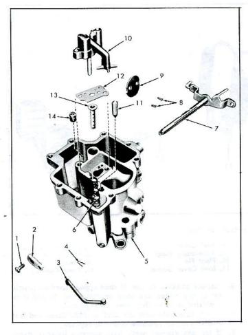
Fig. 21-Carburetor Body-Exploded View
