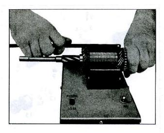
Fig. 5s-Armature Short Circuit Test
