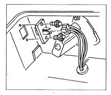
Fig. 6-Resistor Installation
