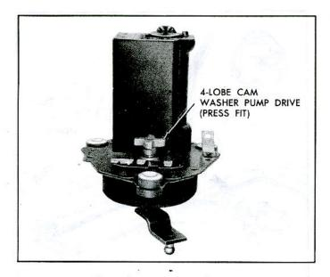
Fig. 31-Washer Pump Drive Cam Location
