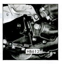
Fig. 3—Differential Number Stamped Lower Left Side of Casting
