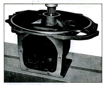
Fig. 42—Pressing Stator Shaft and Pinion Rear Bearing
