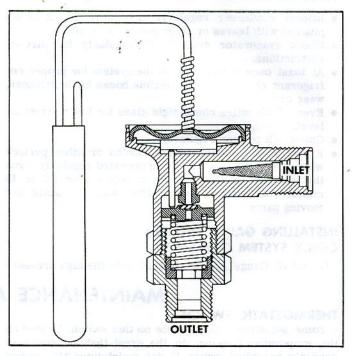
Fig. 19—Expansion Valve Cross Section
