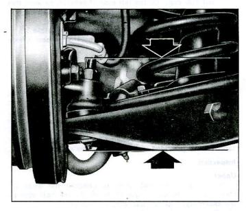
Fig. 3-11-Checking Lower Spherical Joint
