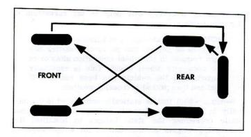
Fig. 6-Tire Rotation Plan
