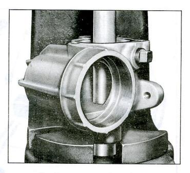
Fig. 11-Removing Sector Shaft Bushing
