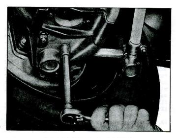
Fig. 3-13-Removing Strut Rod Nut
