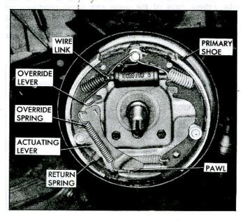
Fig. I-Self-Adjusting Brakes
