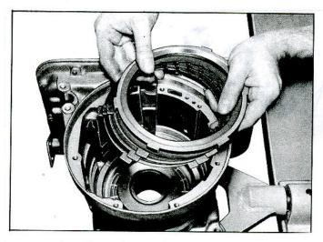
Fig. 7E-26-Removing Reverse Clutch Plates
