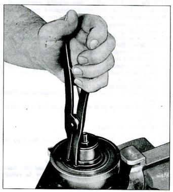
Fig. 37—Removing Coil Housing Retainer Ring
