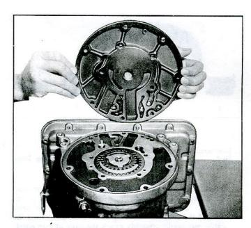
Fig. 7E-20-Removing Front Pump Cover
