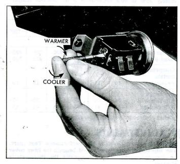
Fig. 18—Thermostatic Switch Adjustment
