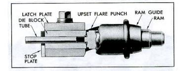
Fig. 11-Flaring Operation-First Flare
