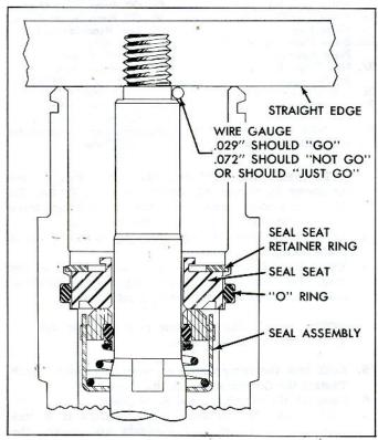
Fig. 40-Checking for Wobble Plate Position on Shaft
