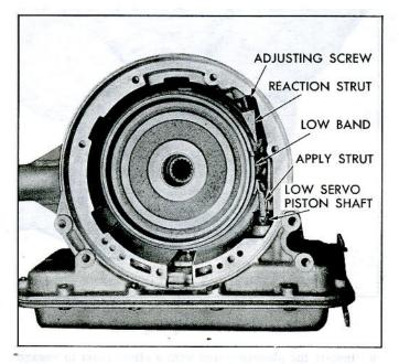
Fig. 7E-55—Low Band Components Installed
