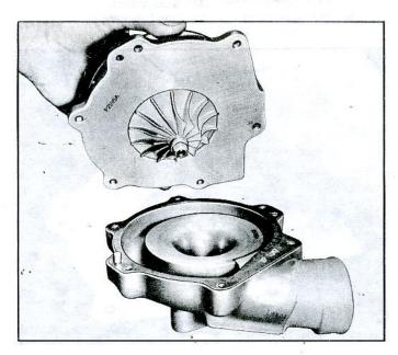
Fig. 39-Removing Compressor Housing
