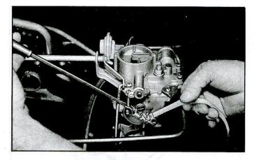
Fig. 7-Adjusting Idle Speed Screw
