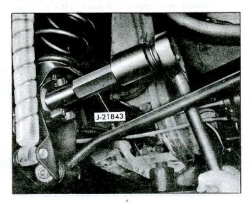
Fig. 67-Installing Wheel Drive Spindle Flange
