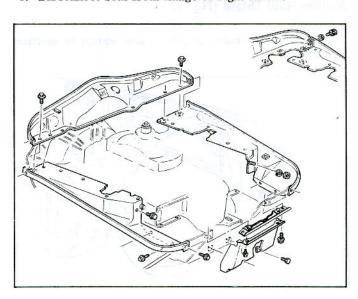
Fig. 21-Engine Shields
