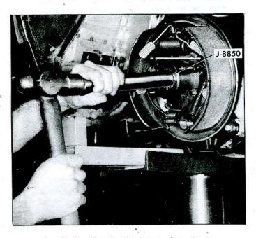
Fig. 70—Installing Spindle Support Outer Bearing
