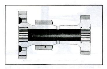
Fig. 7A-21—Countergear Bearings Installed
