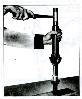
Fig. 21—Installing Pinion Rear Bearing with J-5590
