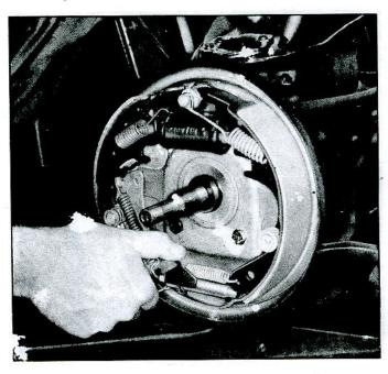
Fig. 21-Checking Operation of the Actuating Lever
