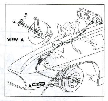
Fig. 26-Speedometer Shaft Assembly
