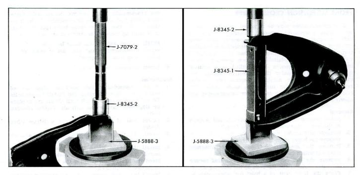
Fig. 3-23—Installing Upper Control Arm Bushings
