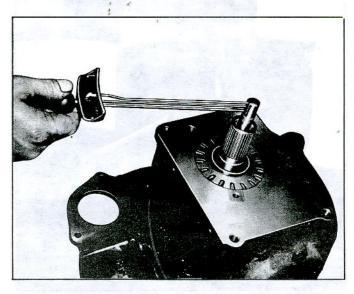
Fig. 48—Measuring Pinion Turning Torque Using J-8362 Adaptor and Torque Wrench J-5853
