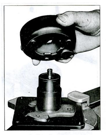
Fig. 38-Installing Coil Housing
