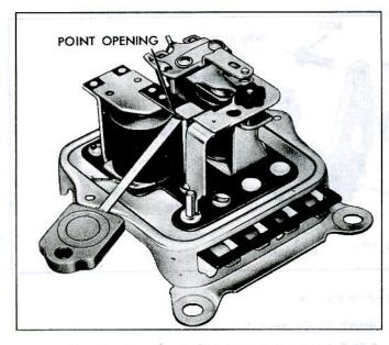
Fig. 23c-Checking Field Relay Point Opening
