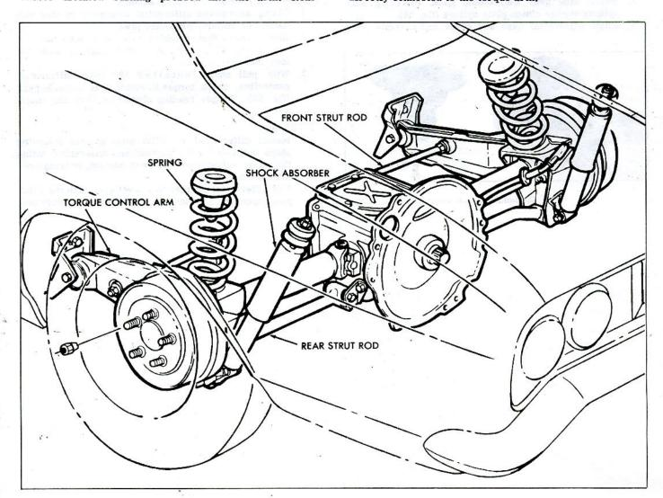
Fig. 60-Rear Suspension Components
