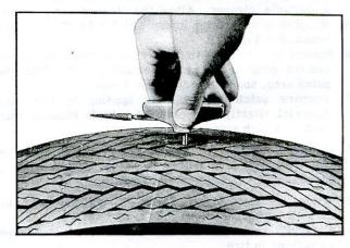
Fig. 14-Making Circular Cut with Reaming Tool
