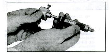
Fig. 20-Measuring Gauge J-6266-19 with Micrometer
