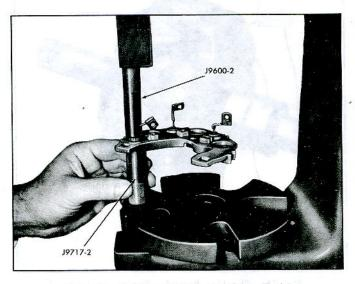
Fig. 19c-Installing Diodes with Press Tools
