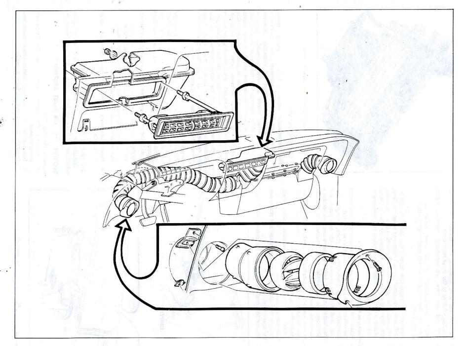
Fig. 25—Air Ducts and Outlets
