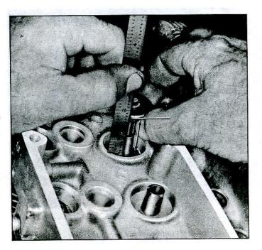
Fig. 38-Measuring Valve Spring Installed Height
