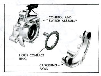
Fig. 27-Direction Signal Control
