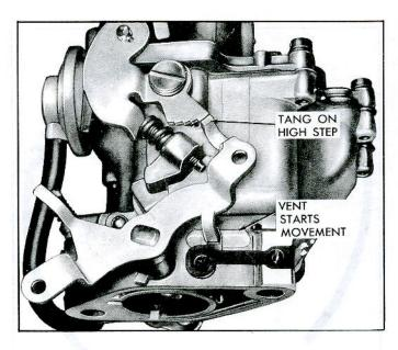
Fig. 14-Vapor Vent Adjustment
