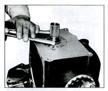
Fig. 47-Tightening Pinion Bearing Adjusting Sleeve with J-972
