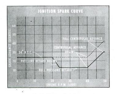
Fig. 1i-Distributor Spark Curve
