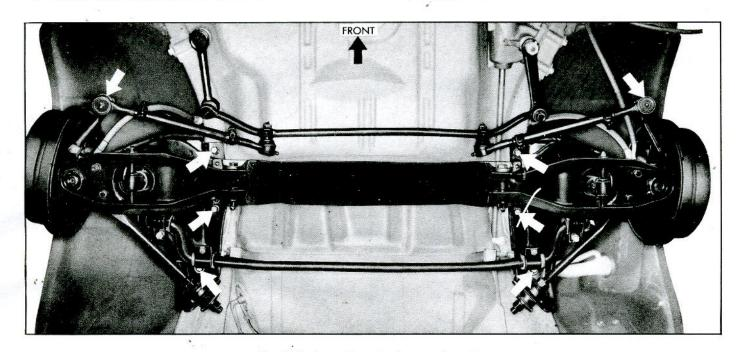
Fig. 3-24-Front Cross Member Attaching Points
