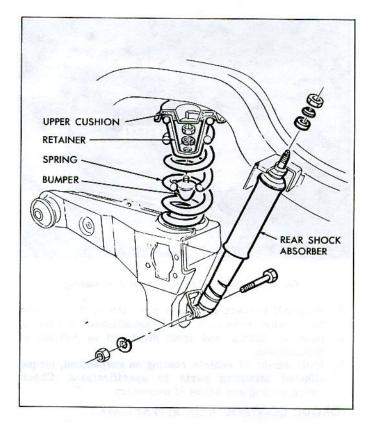
Fig. 79-Spring and Shock Absorber Installation
