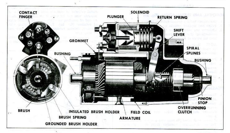
Fig. 1s—Starting Motor Cross Section (Typical)
