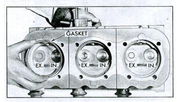
Fig. 69—Cylinder Head Gasket Installation
