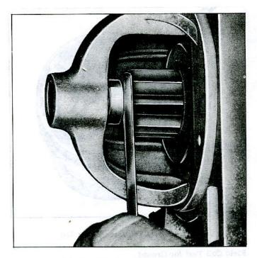
Fig. 11s-Checking Pinion Clearance
