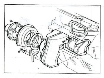
Fig. 26-Blower and Air Inlet Assembly
