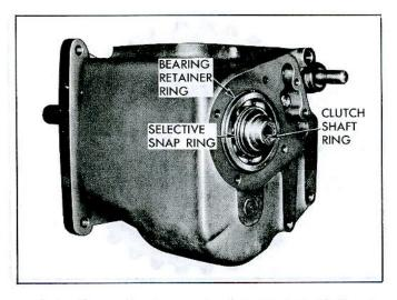
Fig. 7B-21-Clutch Gear and Bearing Snap Rings
