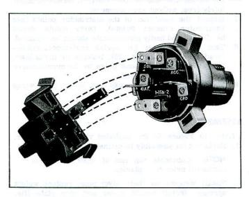
Fig. 10i-Switch and Connector Unplugged
