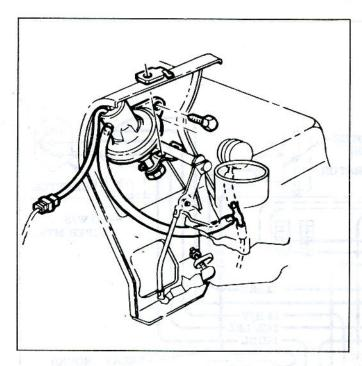
Fig. 58-Fast Idle Adjustment
