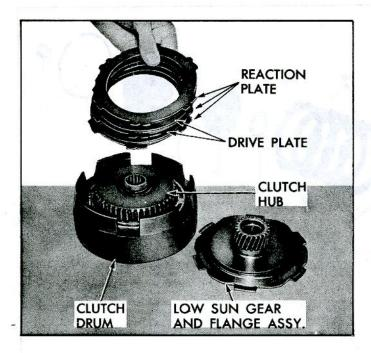
Fig. 7E-37-Installing Clutch Drum Plates
