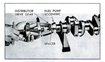
Fig. 119-Removing Distributor Gear
