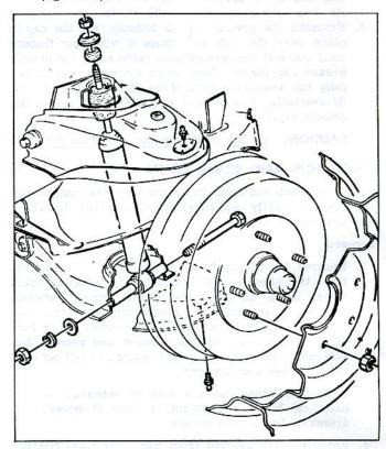
Fig. 3-10-Shock Absorber Installation
