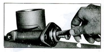
Fig. 23-Checking Main Cylinder Piston Fit
