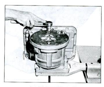
Fig. 7E-18-Removing Front Pump Bolts
