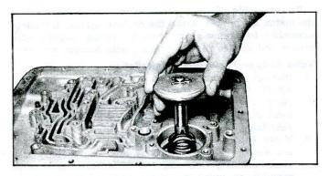
Fig. 7E-14—Installing Low Servo Piston and Return Spring
