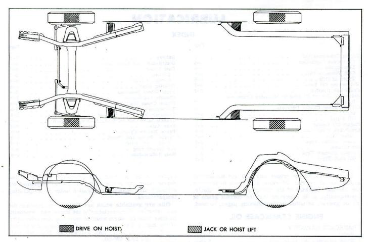
Fig. 16-Lifting Point Diagram
