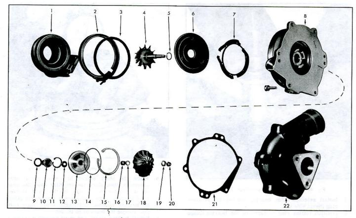
Fig. 44—Turbocharger—Exploded View
