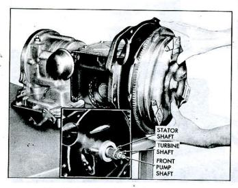
Fig. 12-Installing Converter on Transaxle
