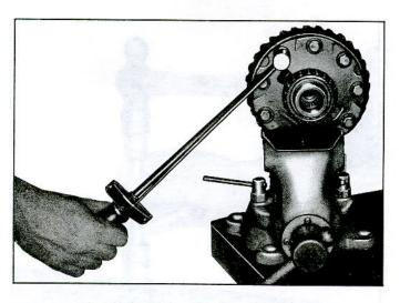
Fig. 35-Measuring Ring Gear Bolt Torque
