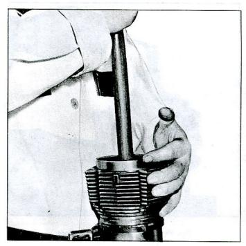
Fig. 97-Removing Piston from Cylinder
