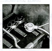
Fig. 9—Battery Number Stamped on Top of the First Cell Adjacent to Positive Terminal
