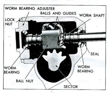
Fig. 1-Steering Gear Worm and Ball Nut Circuits
