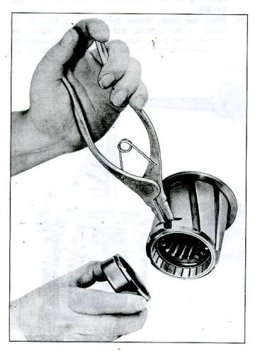
Fig. 7A-15—Removing Synchronizer Ring with J-932
