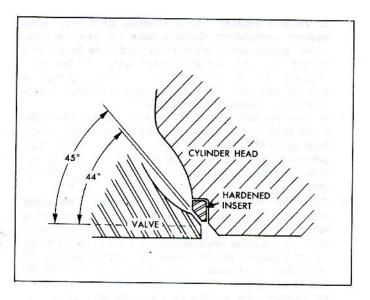
Fig. 85—Relation of Valve and Seat Angles
