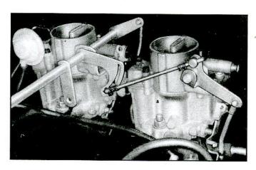
Fig. 19-Rochester H Carburetor Installed
