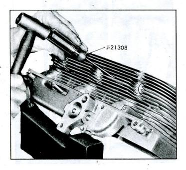
Fig. 84-Cleaning Cooling Fins
