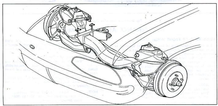
Fig. 3-1-Front Suspension
