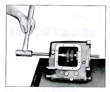
Fig. 7B-8-Removing Countergear Shaft with Dummy Shaft
