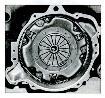
Fig. 7-5-Clutch Assembly Installed
