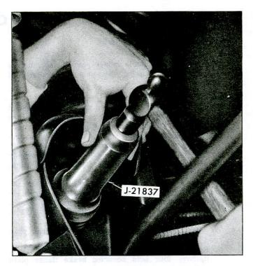
Fig. 68-Installing Spindle Support Inner Seal
