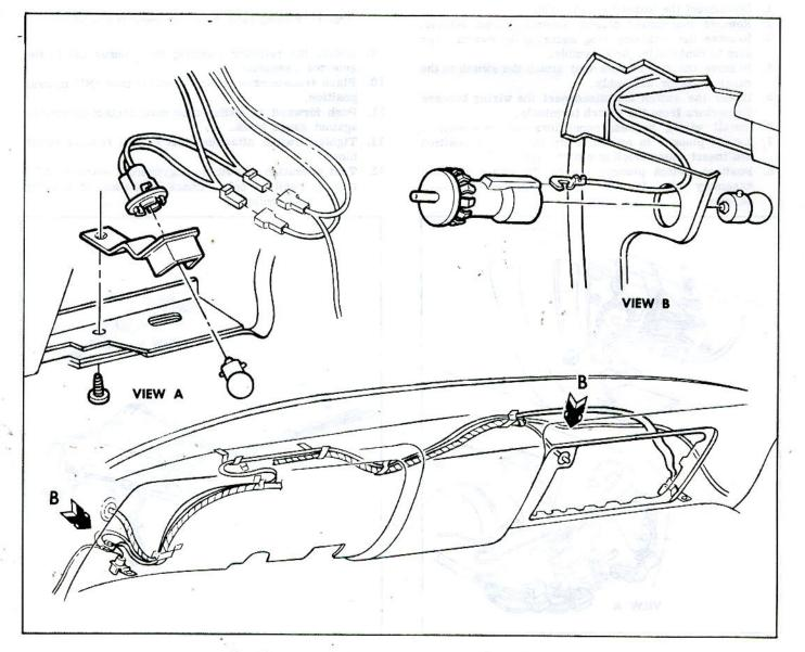
Fig. 20-Instrument Panel Compartment and Courtesy Lamps
