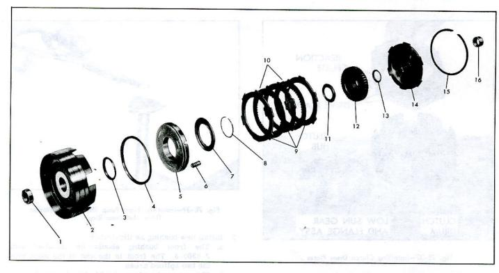
Fig. 7E-35-Clutch Drum-Exploded View
