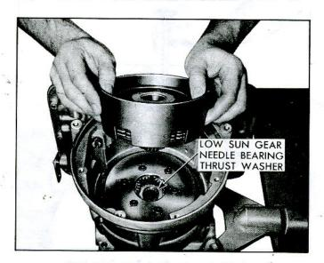
Fig. 7E-23-Removing Clutch Drum
