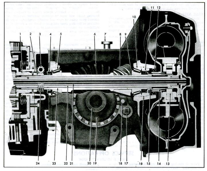
Fig. 2-Automatic Transmission Rear Axle
