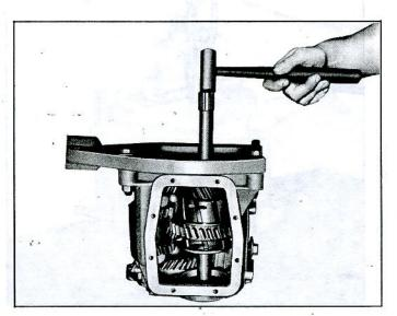
Fig. 7A-8-Driving Mainshaft from Transmission
