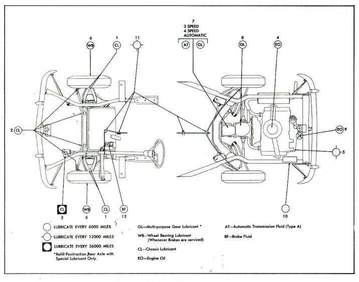
Fig. 17-Corvair Lubrication Diagram
