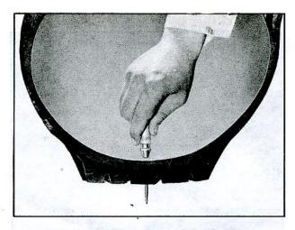
Fig. 11-Installing Needle in Tire Hole
