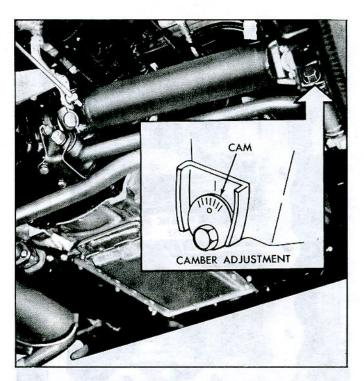
Fig. 44-Rear Strut Rod and Cam Adjustment
