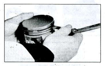
Fig. 106-Measuring Ring Groove Clearance
