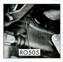
Fig. 8–3—and 4–Speed Transmission Unit Numbers Stamped on a Boss on L.H. Side of Transmission Above Shifter Shaft Outlet
