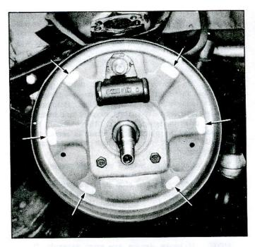
Fig. 20-Backing Plate Contact Surfaces
