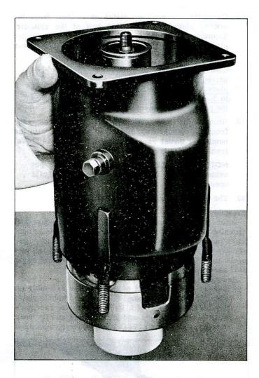
Fig. 56-Installing Shell Over Internal Mechanism
