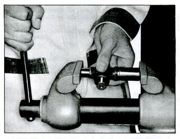
Fig. 5-"U" Joint Trunnion Seal Installation
