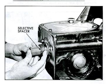
Fig. 7-Removing Governor Drive Gear and Spacers
