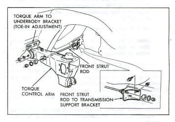
Fig. 77-Front Strut Rod Attachment
