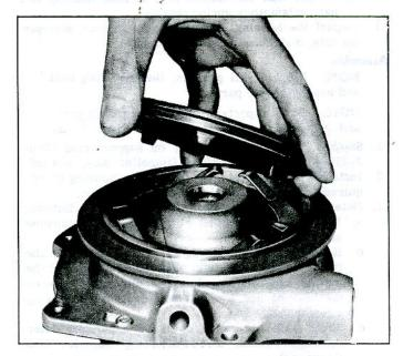
Fig. 48-Heat Shield Spring Ring Installation
