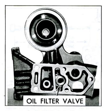
Fig. 111-Oil Filter By-Pass Valve
