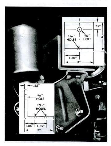
Fig. 49-Lifting Adapter
