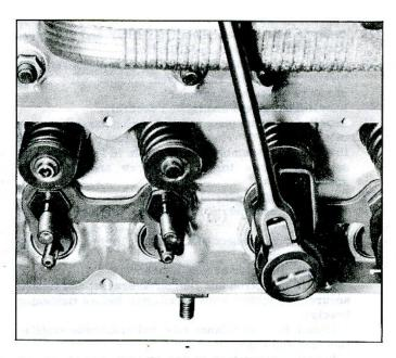
Fig. 74-Push Rods Installed
