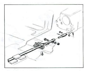
Fig. 7A-3—Control Rod & Linkage
