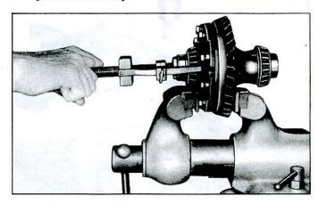
Fig. 28-Removing Differential Side Bearings
