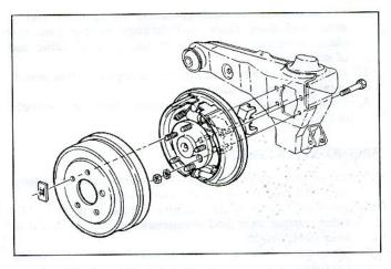
Fig. 82-Rear Wheel Spindle, Support and Brake Removal
