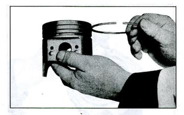
Fig. 105-Rolling Ring in Groove
