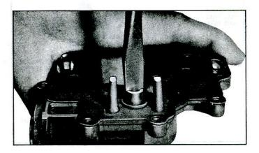
Fig. 5-Removing Needle Seat
