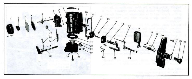
Fig. 27—Carburetor—Exploded View
