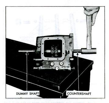
Fig. 7B-17—Installing Countergear Shaft
