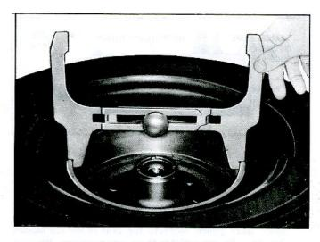
Fig. 13-Using Drum-to-Brake Shoe Clearance Gauge
