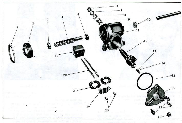
Fig. 8-Exploded View of Steering Gear
