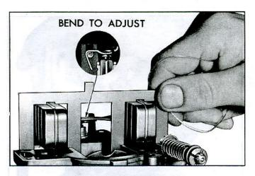
Fig. 11-Checking Float Level
