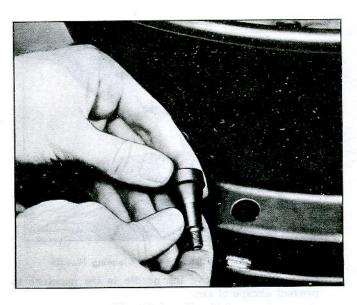
Fig. 22-Installing Valve
