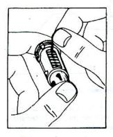
Fig. 14—Inserting Tumbler Springs
