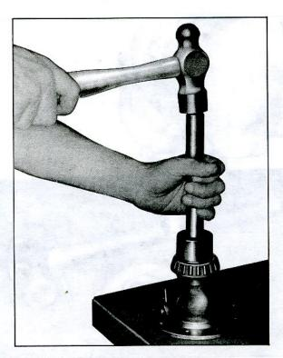
Fig. 31—Installing Differential Side Bearing with J-8359 and J-7079-2 Handle
