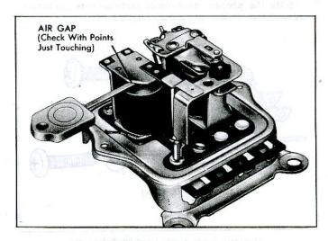
Fig. 24c-Checking Field Relay Air Gap
