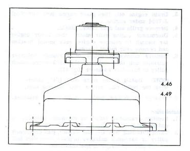
Fig. 29-Blower Bearing Replacement
