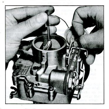
Fig. 13-Vacuum Diaphragm Adjustment
