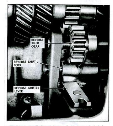
Fig. 7B–18—Installation of Reverse Shifter Lever, Shift Fork, and Reverse Idler Gear
