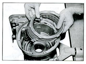
Fig. 7E<sub>7</sub>51—Installing Reverse Clutch Plates
