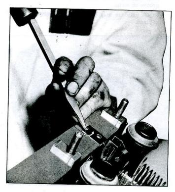
Fig. 92—Choke Coil Removal
