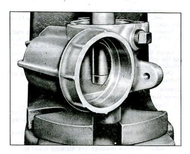
Fig. 12-Installing Sector Shaft Bushing
