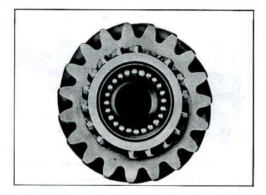
Fig. 7A-27—Mainshaft Pilot Bearings in Clutch Gear
