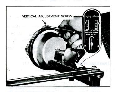
Fig. 5-Headlamp Vertical Adjustment
