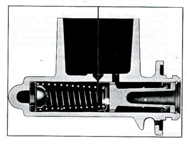
Fig. 24-Checking Compensating Port Clearance
