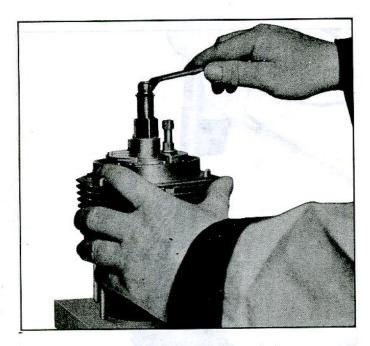
Fig. 99-Removing Ridge from Cylinder
