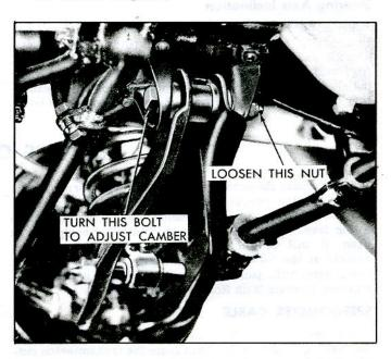
Fig. 3-4-Camber Adjustment
