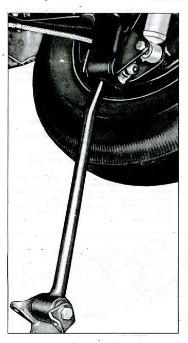
Fig. 45-Rear Strut Rod Lowered
