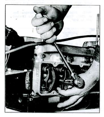
Fig. 77—Adjusting Valves
