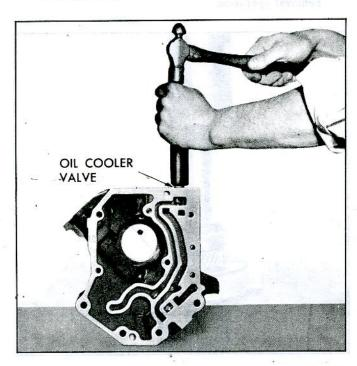
Fig. 115-Installing Oil Cooler By-Pass Valve
