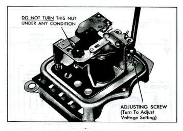
Fig. 4c-Adjust Voltage Setting
