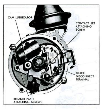
Fig. 2i-Breaker Plate and Attaching Parts
