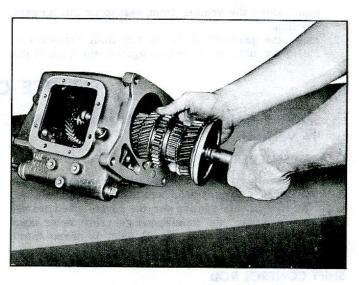
Fig. 7B-6-Removing Assembled Mainshaft Components
