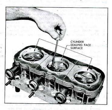
Fig. 81-Cleaning Valve Guides
