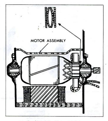
Fig. 34—End Play Washers Installed
