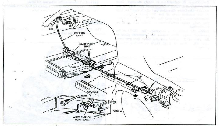
Fig. 7E-5—Shift Control Cable Routing
