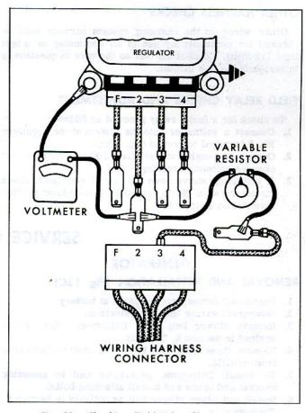
Fig. 11c-Checking Field Relay Closing Voltage
