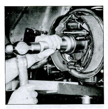
Fig. 74-Installing Spindle Support Outer Seal
