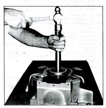
Fig. 118-Installing Flywheel Housing Seal
