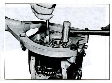
Fig. 7A-9—Removing Mainshaft Bearing from Case
