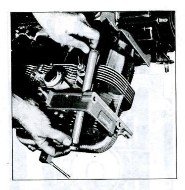
Fig. 70-Installing Push Rod Tubes
