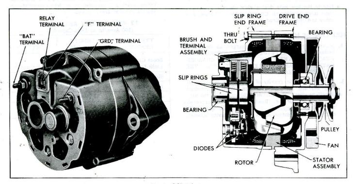
Fig. Ic-5.5" Delcotron
