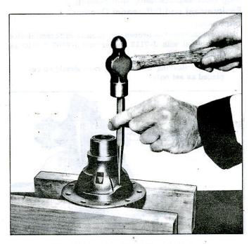
Fig. 30—Removing Pinion Gear Shaft Pin
