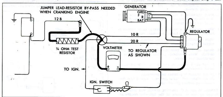
Fig. 5c-Voltage Setting Test Connections
