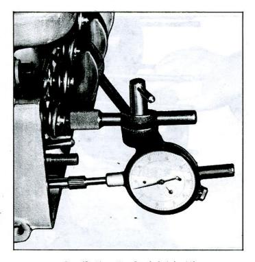
Fig. 42-Measuring Camshaft Lobe Lift
