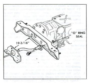
Fig. 7E-6-Cable-to-Case Installation
