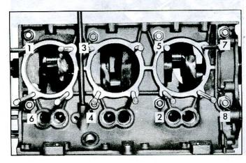
Fig. 59-Crankcase Torque Sequence
