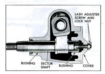
Fig. 4-Sector Gear and Pitman Shaft
