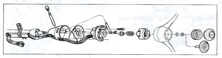
Fig. 17-Exploded View of Mast Jacket and Steering Wheel
