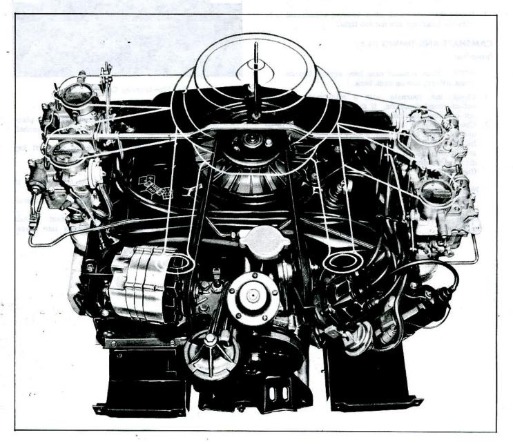
Fig. 127—Corsa Engine (4 x 1 Carburetor)
