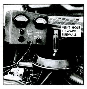
Fig. 64-Tool Installed on Air Cleaner
