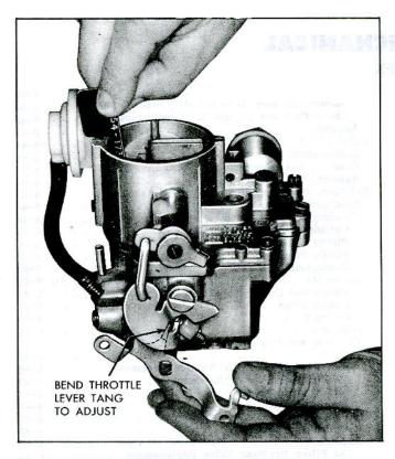
Fig. 16-Choke Unloader Adjustment
