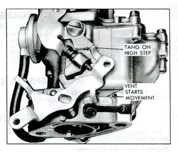
Fig. 17-Vapor Vent Adjustment
