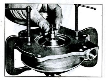
Fig. 52-Shaft Sleeve and Shim Installation
