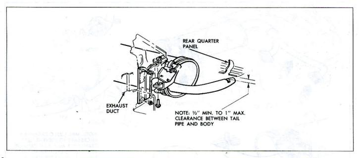
Fig. 8-Muffler and Bracket Attachment
