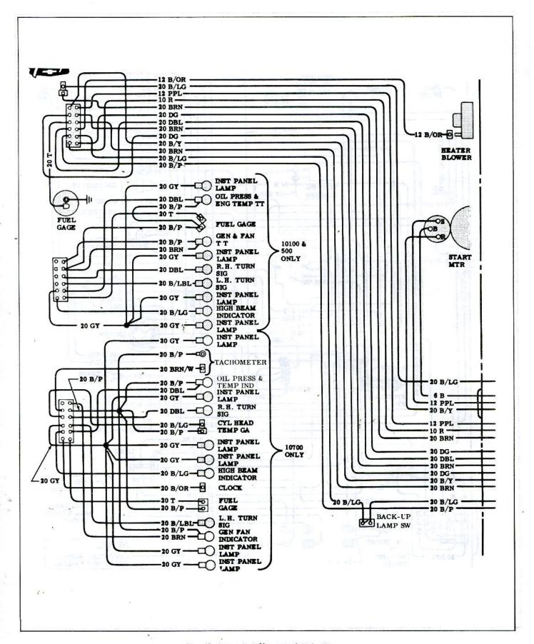
Fig. 48—Instrument Cluster and Body Harness
