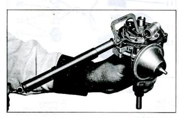
Fig. 3i-Checking Breaker Arm Spring Tension
