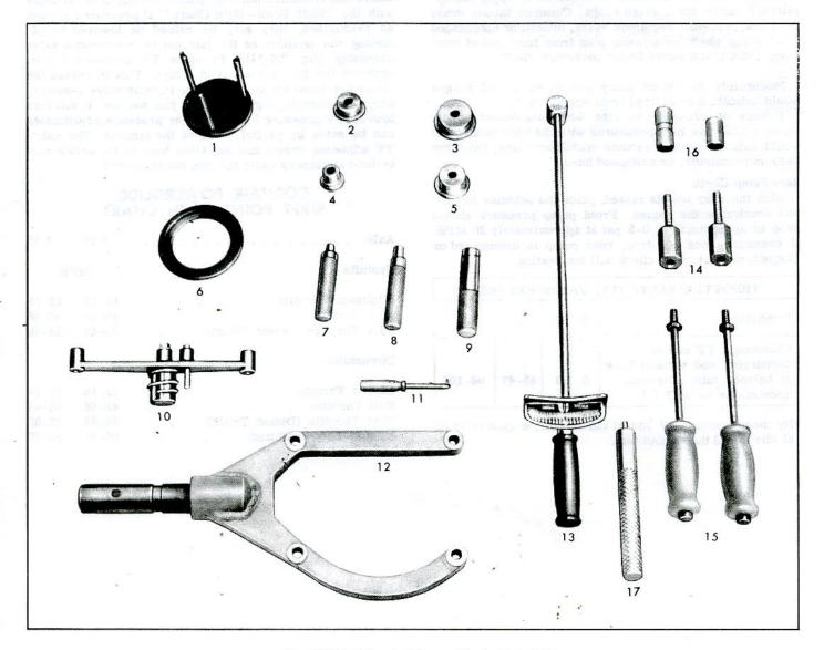
Fig. 7E-63-"Corvair" Powerglide Special Tools
