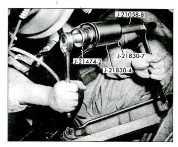
Fig. 80-Removing Torque Control Arm Bushing
