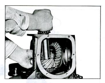
Fig. 16-Removing Pinion from Carrier
