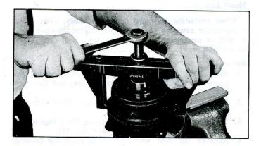
Fig. 36-Removing Pulley
