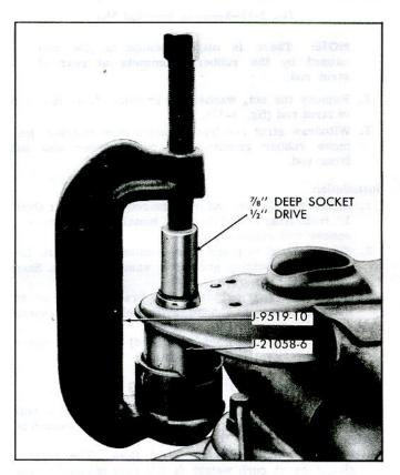
Fig. 3-18-Removing Spherical Joint
