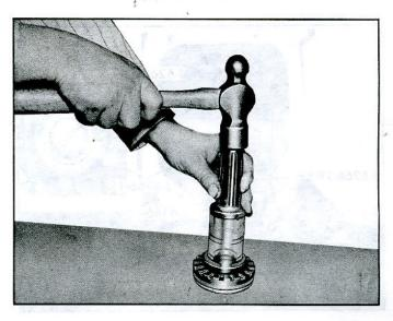
Fig. 24—Installing Pinion Front Oil Seal— Automatic Transmission Only
