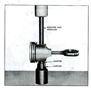
Fig. 98-Removing Piston Pin
