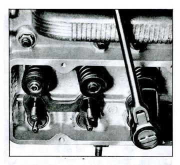
Fig. 35-Push Rods Installed
