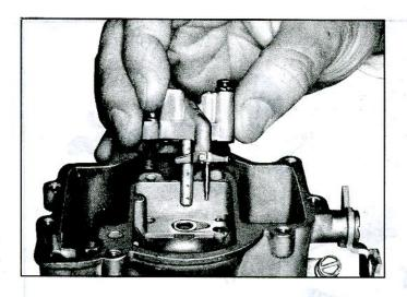
Fig. 6-Removing Venturi Cluster
