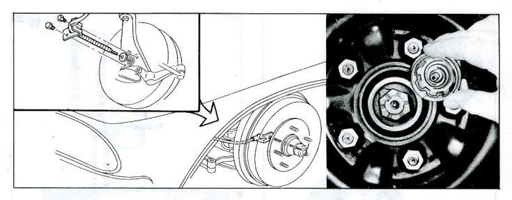
Fig. 3-6-Speedometer Cable
