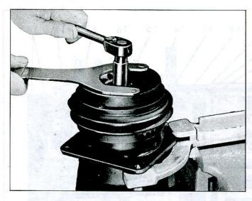
Fig. 31-Removing Shaft Locknut
