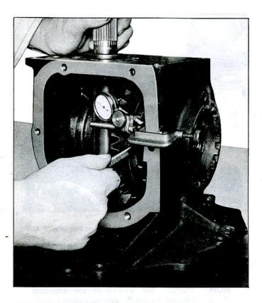
Fig. 49—Measuring Ring Gear-to-Pinion Backlash with J-8001
