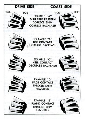
Fig. 52-Ring Gear Contact Patterns
