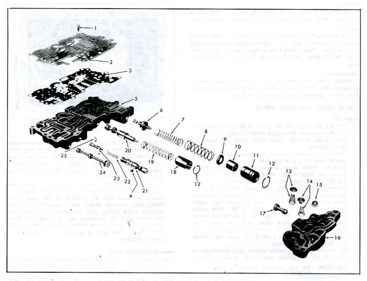
Fig. 7E-11—Corvair Powerglide Valve Body—Exploded View
