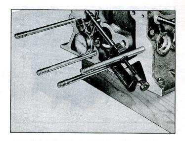
Fig. 61-Measuring Camshaft End Play
