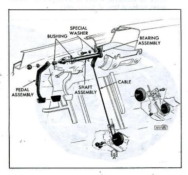
Fig. 7-8-Clutch Pedal and Cable
