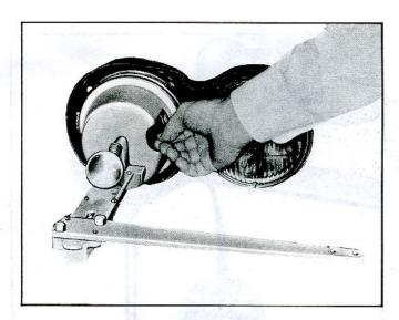
Fig. 6-Removing Aimer from Headlamp
