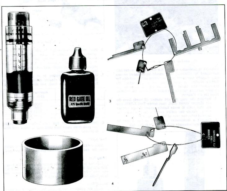
Fig. 67-Engine Fuel Special Tools
