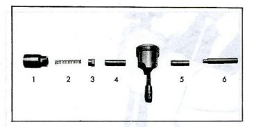
Fig. 101—Piston Assembly and Tool Layout
