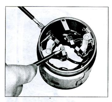
Fig. 7s-Field Coil Open Circuit Test
