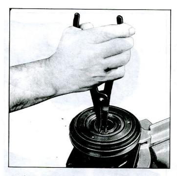
Fig. 35-Removing Pulley and Bearing Assembly Retainer Ring
