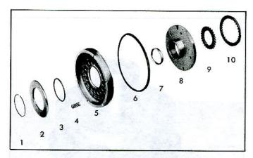
Fig. 7E-40—Rear Pump and Reverse Piston—Exploded View
