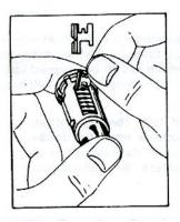
Fig. 12—Inserting Tumblers
