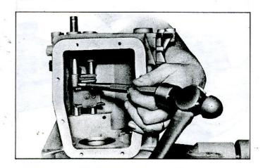
Fig. 7A-20-Installing Second and Third Shift Fork
