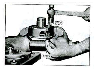
Fig. 7E-47-Installing Long Planet Pinion
