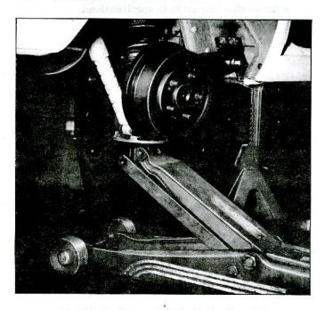
Fig. 78—Positioning Jack for Spring Removal
