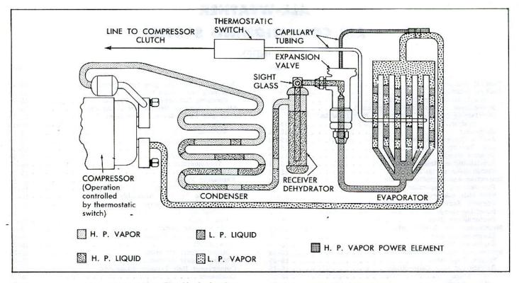
Fig. 10-Cycle of Operation-Corvair Air Conditioning
