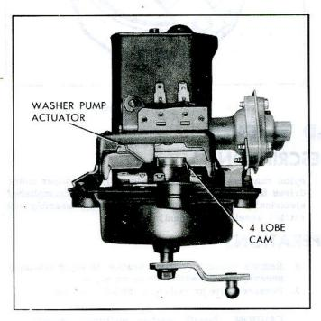
Fig. 38-Washer Drive Mechanism
