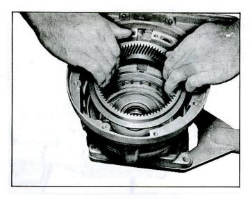
Fig. 7E-24—Removing Ring Gear
