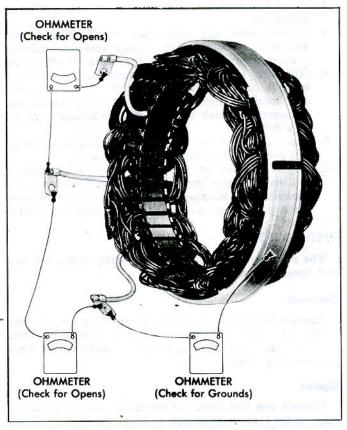
Fig. 17c—Checking Stator for Grounds or Opens
