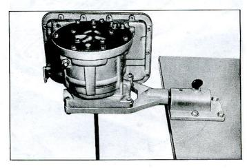
Fig. 7E-17—Transmission in Holding Fixture J-7896
