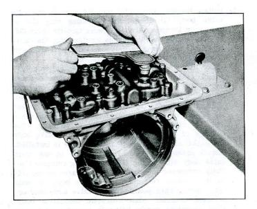
Fig. 7E-16—Installing Valve Body Screen
