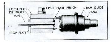
Fig. 10-Flaring Operation-Positioning Tubing
