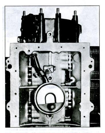
Fig. 68-Oil Pick-Up Screen Installed
