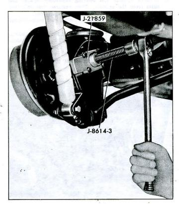
Fig. 64-Removing Wheel Spindle Flange
