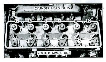
Fig. 73-Cylinder Head Torque Sequence
