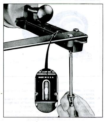
Fig. 8-Turning Level Adjusting Screw to Calibrate Aimer
