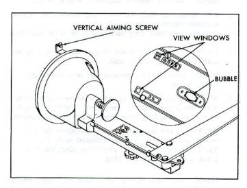
Fig. 7-Selecting Level Aiming Area
