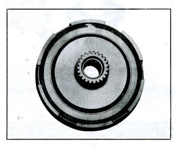
Fig. 7E-38—Clutch Flange and Low Sun Gear Retainer Ring Installation
