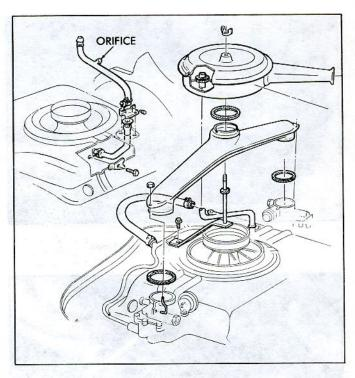
Fig. 5-Crankcase Ventilation
