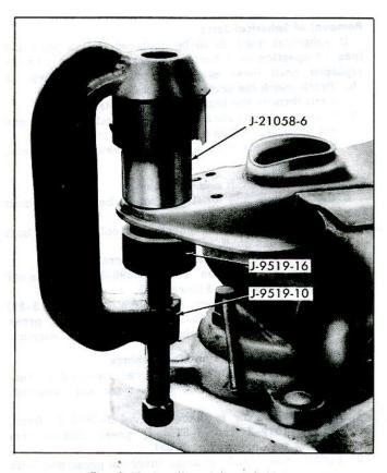
Fig. 3-19—Installing Spherical Joint
