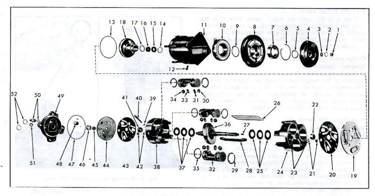
Fig. 39-Six-Cylinder Compressor-Exploded View
