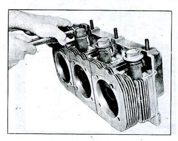
Fig. 86-Removing Exhaust Manifold Sleeves
