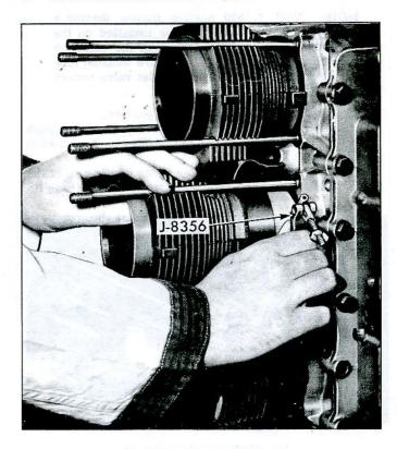
Fig. 41-Removing Tool from Piston Assembly
