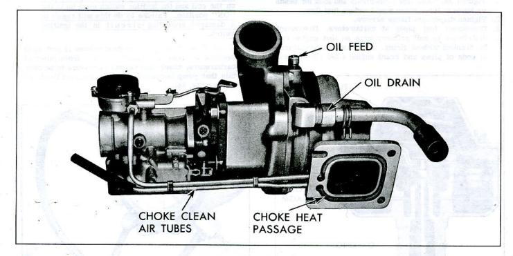
Fig. 56-Turbocharger Fittings and Passages
