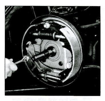
Fig. 19—Removing Hold Down Springs and Pins
