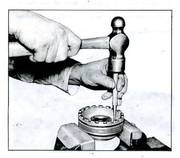
Fig. 26-Removing Side Bearing Race
