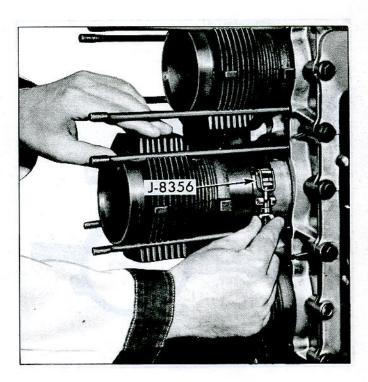
Fig. 40-Compressing Piston Rings
