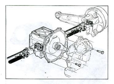
Fig. 3-Axle Drive Shaft Installation
