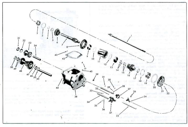
Fig. 7A-13—Manual Transmission—Exploded View
