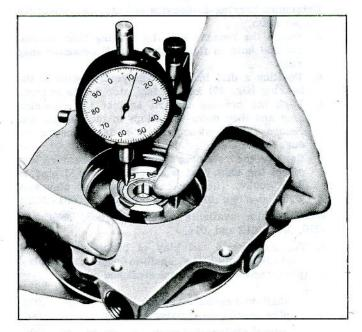
Fig. 46-Gauging Bearing-to-Housing End Play
