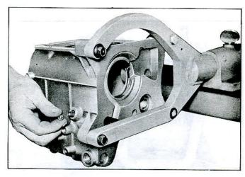
Fig. 7A-17—Installing Detent Spring and Ball for First and Reverse Shift Fork Shaft
