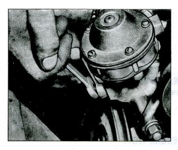
Fig. 59-Loosening Locknut
