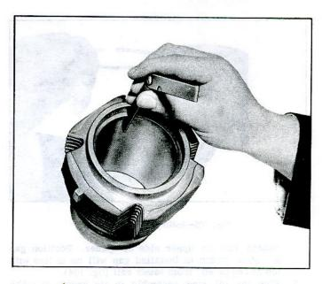
Fig. 103-Measuring Ring Gap
