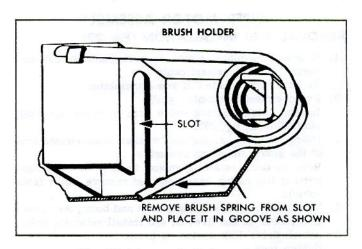
Fig. 33—Releasing Brush Spring Tension
