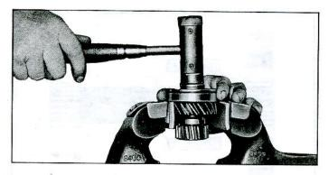
Fig. 7A-14-Removing Clutch Gear Bearing
