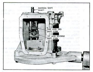
Fig. 7A-11—Shift Forks Installed
