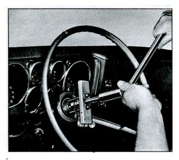
Fig. 6-Steering Wheel Removal
