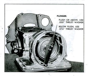
Fig. 7E-56—Gauging Clutch Drum Thrust Washer with J-8371
