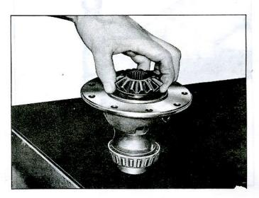
Fig. 32-Installing Side Gear in Differential Case
