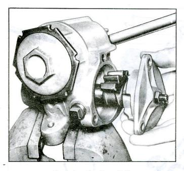
Fig. 9-Removing Pitman Shaft
