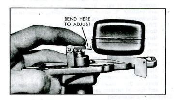
Fig. 31—Adjusting Float Level
