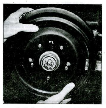
Fig. 15-Aligning Drum Tang with Wheel Hub
