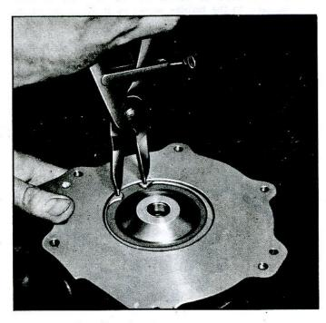
Fig. 42-Oil Seal Retainer Ring Removal
