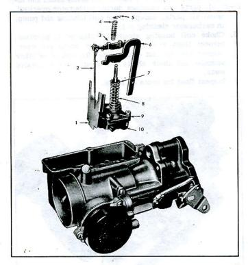
Fig. 29-Pump and Metering Rod Assembly
