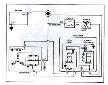
Fig. 2c-Two Unit Voltage Regulator
