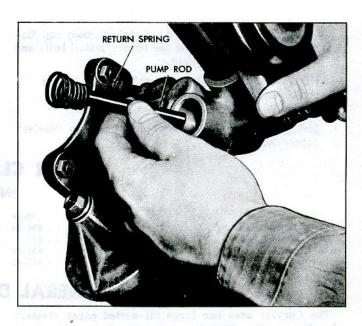
Fig. 60-Removing Push Rod
