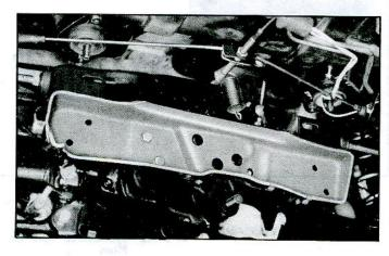
Fig. 7B-24-Removing Manual Transmission from Vehicle
