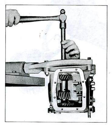
Fig. 7A-22-Installing Countershaft in Countergear
