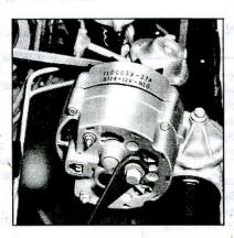
Fig. 5—Delcotron Information Located on Drive End Frame
