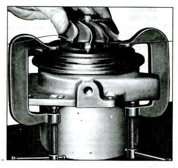
Fig. 51-Installation of Turbine Wheel and Shaft
