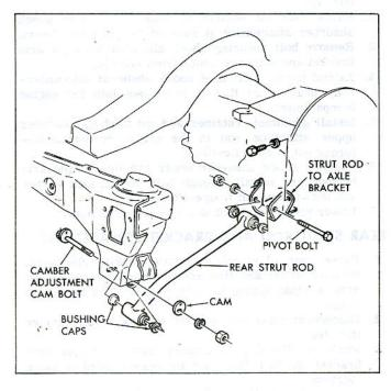
Fig. 76-Rear Strut Rod Attachment
