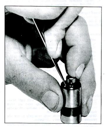
Fig. 95-Installing Ball Check Valve
