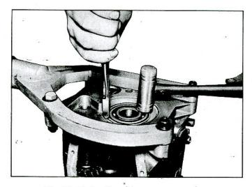
Fig. 7A-24-Installing Mainshaft Rear Bearing
