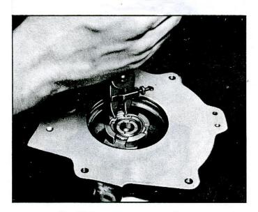
Fig. 43-Removing Bearing Retainer Ring
