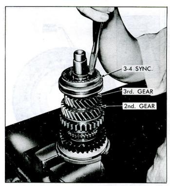
Fig. 7B-9-Mainshaft Front Components
