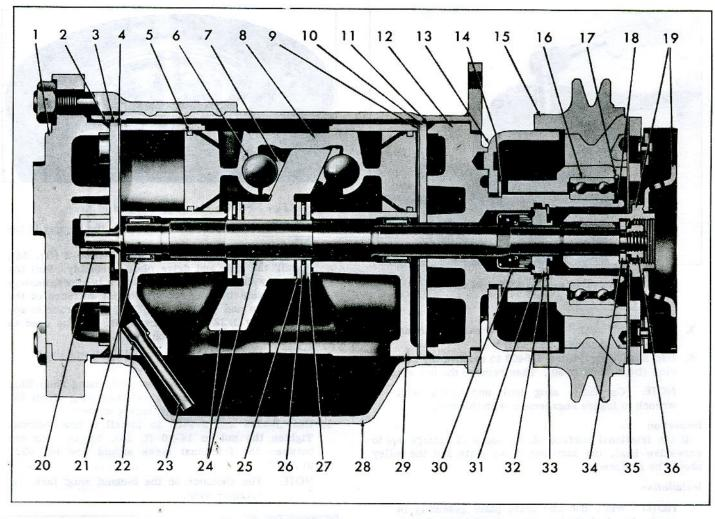
Fig. 30-Six-Cylinder Compressor-Cross Section View
