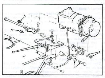
Fig. 29-Compressor Mounting
