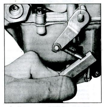
Fig. 24-Adjusting Pump Rod
