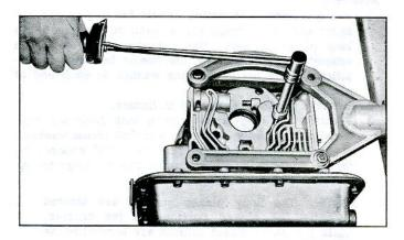
Fig. 7E-50-Measuring Rear Pump and Reverse Piston Bolt Torque
