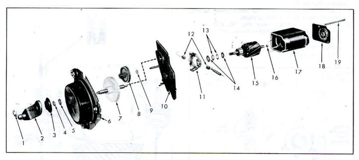
Fig. 30-Wiper Motor and Gear Box Exploded View (Typical)
