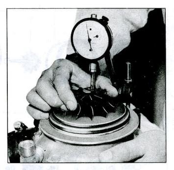
Fig. 47-Gauging Impeller-to-Housing Clearance
