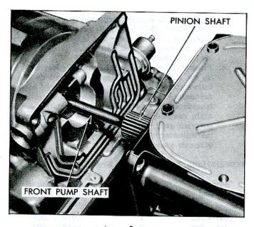
Fig. 11—Engaging Pinion Shaft-to-Transmission Planet Carrier Splines
