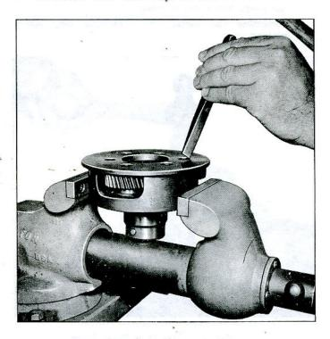
Fig. 7E-48-Staking Planet Pinion Shaft
