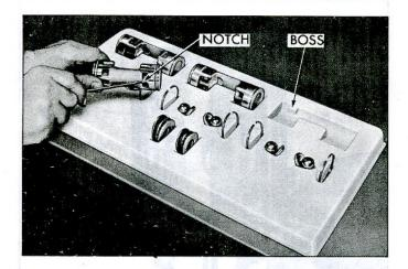
Fig. 49-Notch Identifying Front End of Piston
