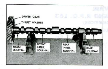
Fig. 125-Checking Camshaft Alignment
