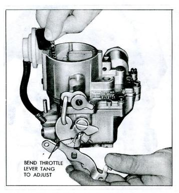
Fig. 15-Choke Unloader Adjustment
