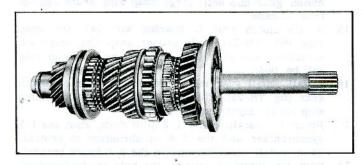
Fig. 7B-16—Assembled Mainshaft
