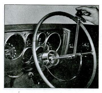
Fig. 5-Checking Steering Gear Turning Torque
