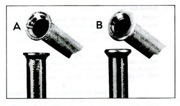
Fig. 9-Single and Double Lap Flaring
