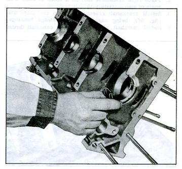
Fig. 55-Removing Main Bearings
