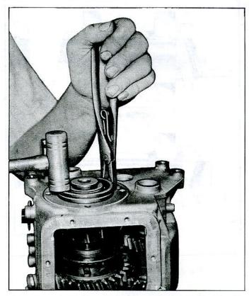
Fig. 7A-28—Installing Clutch Gear Bearing
