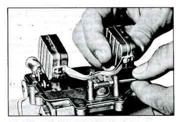
Fig. 10-Replacing Floats
