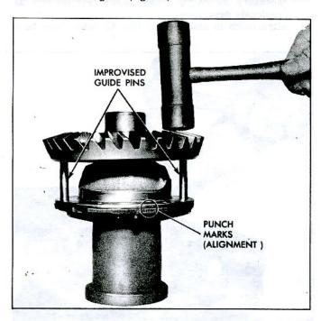
Fig. 34—Installing Ring Gear on Differential Case and Cover
