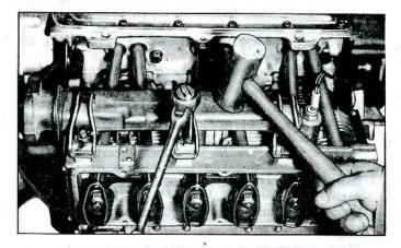
Fig. 75-Installing Exhaust Manifold
