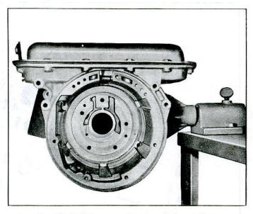
Fig. 7E-49—Transmission Case Installed in Holding Fixture J-7896
