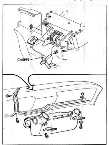
Fig. 23-Evaporator Removal
