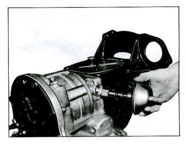
Fig. 6-Removing Governor
