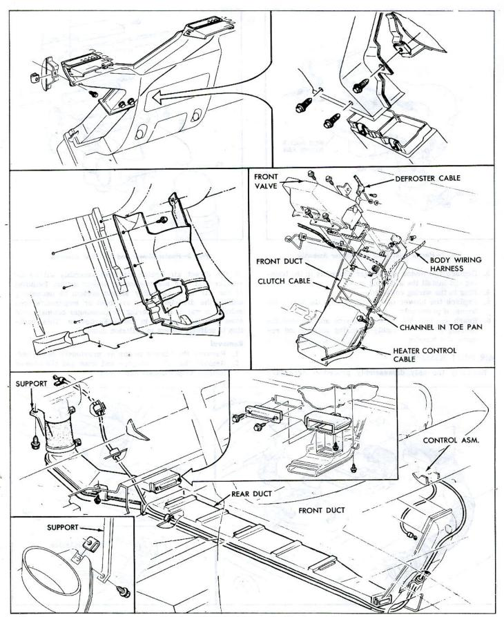
Fig. 5-Heater Air Ducts
