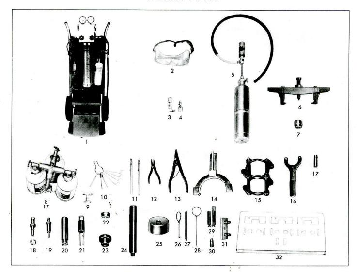
Fig. 61-Air Conditioning Special Tools
