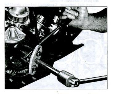
Fig. 53-Removing Harmonic Balancer
