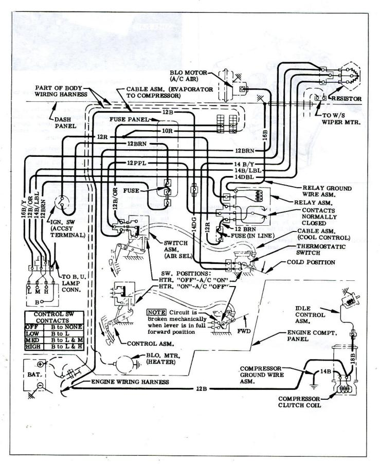
Fig. 60-Air Conditioning Wiring Diagram
