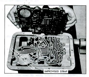
Fig. 7E-10-Removing Valve Body
