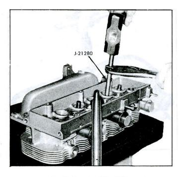
Fig. 88-Removing Valve Guide
