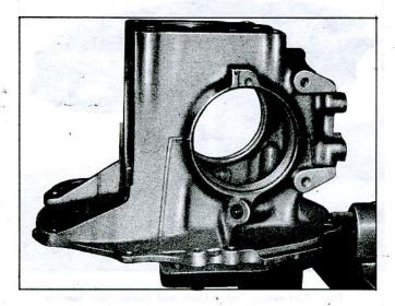
Fig. 44-Differential Carrier Installed in J-3289 Holding Fixture
