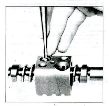
Fig. 13-Installing Balls in Nut
