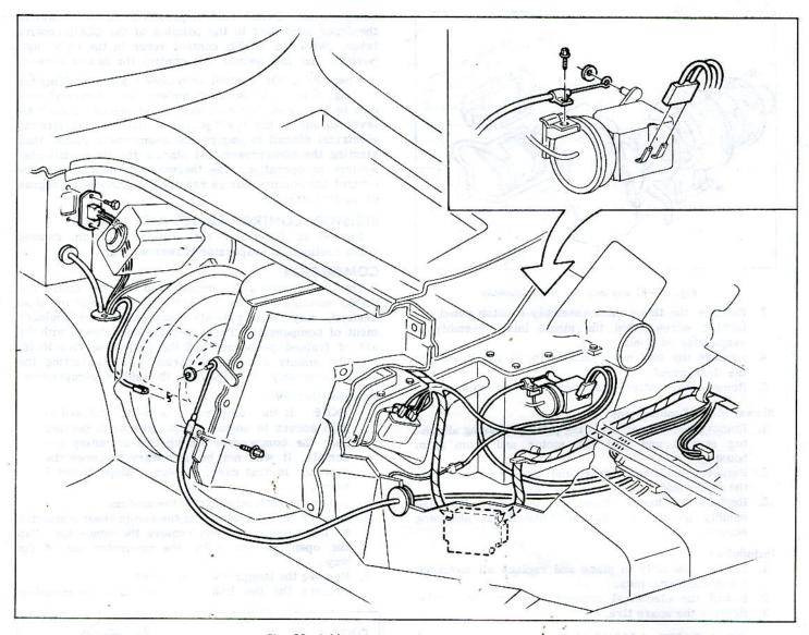
Fig. 28-Cables, Wiring and Resistor Location
