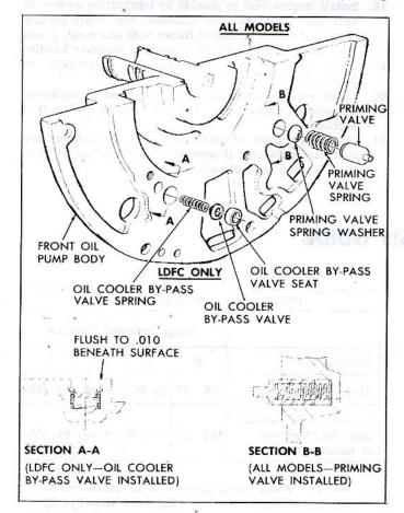
Fig. 7E-60-Front Pump Body and Components
