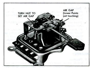
Fig. 22c-Checking Voltage Regulator Air Gap
