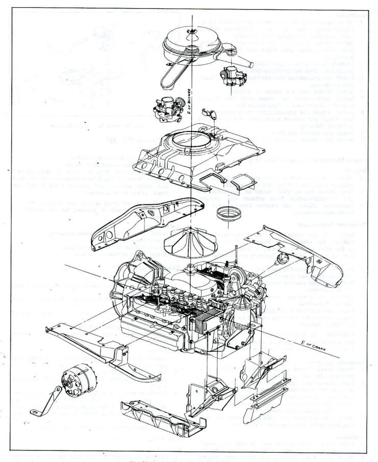
Fig. 25-Engine Sheet Metal-Exploded View
