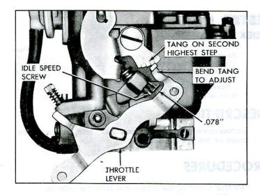
Fig. 16—Fast Idle Adjustment
