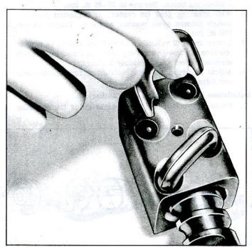
Fig. 15-Inserting Ball Guides in Nut
