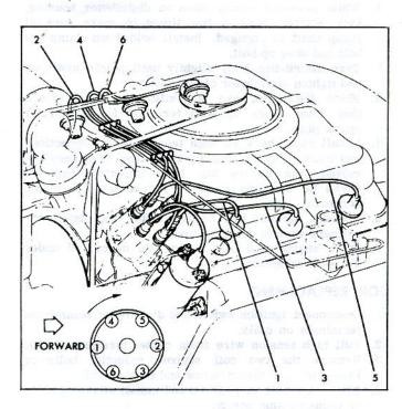
Fig. 8i-Distributor, Spark Plug Wires Installed
