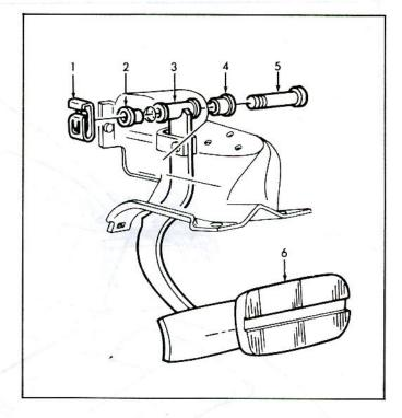
Fig. 17-Brake Pedal and Attachments-w/Automatic Trans.
