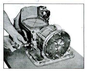
Fig. 7E-8-Removing Vacuum Modulator and Valve
