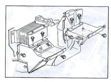
Fig. 30-Oil Cooler and Exhaust Ducts
