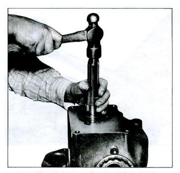
Fig. 37—Installing Pinion Shaft Front Seal with J-8340
