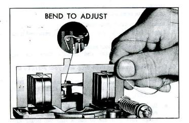
Fig. 22-Checking Float Level
