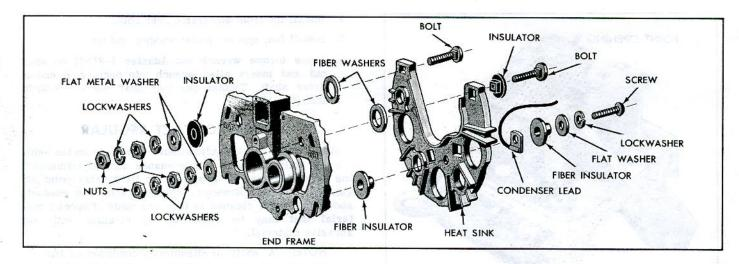
Fig. 20c—Heat Sink—Parts Location
