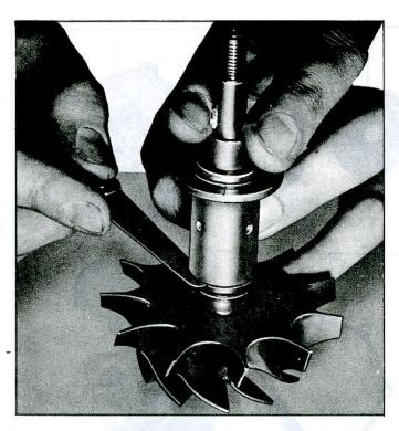
Fig. 45-Measuring Bearing-to-Shaft End Play
