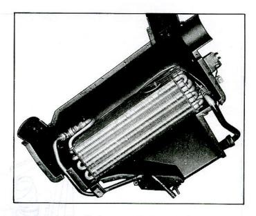
Fig. 24-Evaporator Cover Removed
