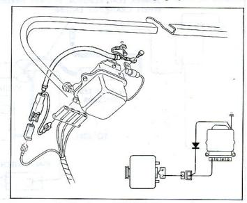
Fig. 3c-External Field Discharge Diode
