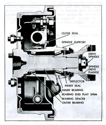
Fig. 66-Wheel Spindle and Support Cross Section
