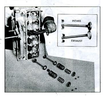
Fig. 79-Compressing Valve Springs
