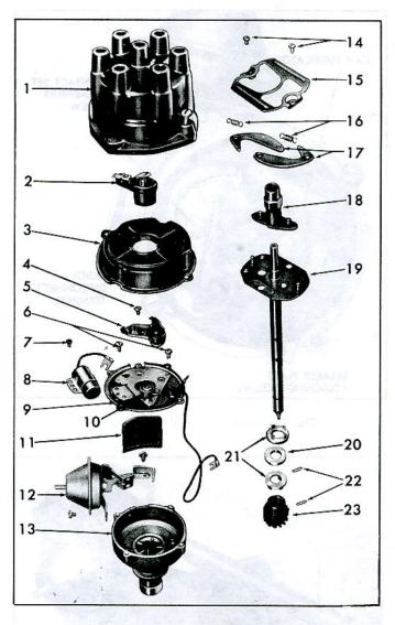
Fig. 6i-Distributor Exploded View
