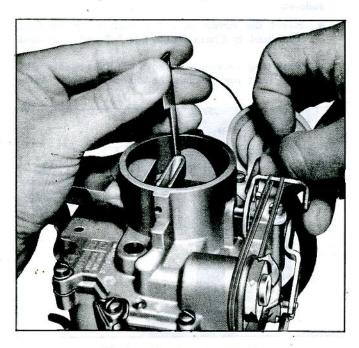
Fig. 14-Vacuum Diaphragm Adjustment
