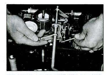
Fig. 130—Synchronization of Secondary Carburetor
