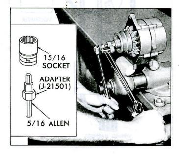
Fig. 15c-Torquing Pulley Nut
