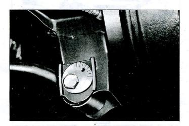
Fig. 61-Camber Adjusting Cam Location
