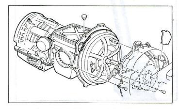
Fig. 48-Transaxle Separated from Engine
