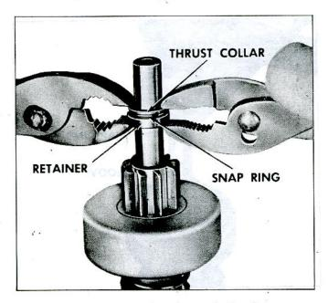
Fig. 10s-Forcing Snap Ring into Retainer
