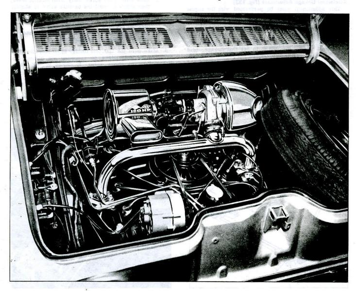
Fig. 132—Turbocharged Engine (Installed)
