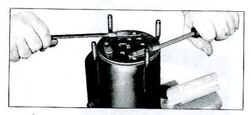
Fig. 43—Removing Rear Discharge Valve Plate
