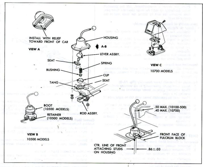
Fig. 7A-2-Gearshift Lever Assembly-Exploded View
