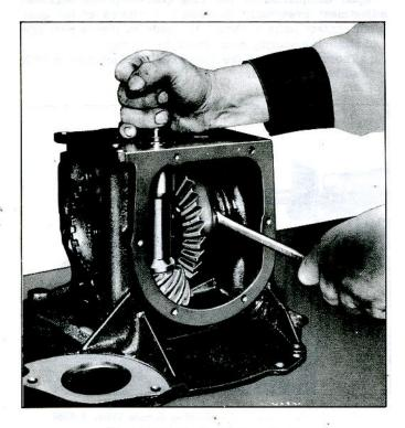
Fig. 50-Developing Contact Pattern
