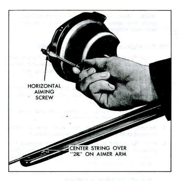
Fig. 4-Headlamp Horizontal Adjustment
