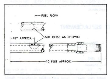
Fig. 5-Siphon Construction
