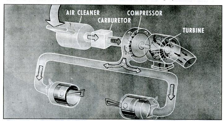
Fig. 35-Turbocharger Operational Schematic
