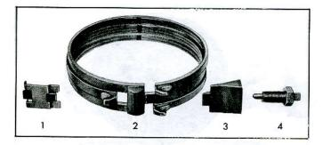
Fig. 7E-22—Low Band Components
