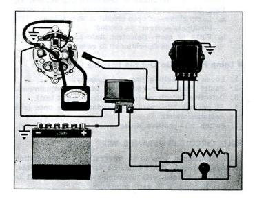
Fig. 6c—Output Test Connections (Typical)
