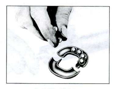
Fig. 14—Filling Ball Guides
