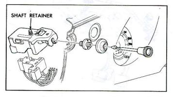
Fig. 11-Lighting Switch Installation
