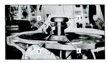
Fig. 7-4-Removing Clutch Release Bearing
