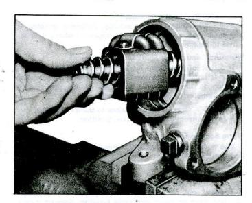
Fig. 10-Removing Wormshaft and Ball Nut
