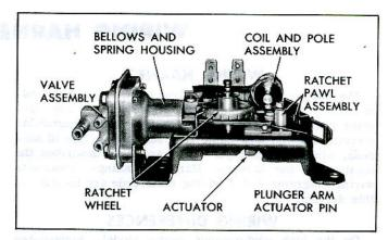
Fig. 37-Washer Pump Mechanism
