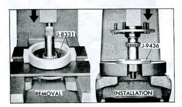
Fig. 72—Removing and Installing Drive Spindle Outer Bearing
