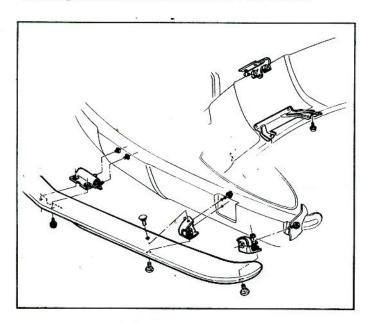
Fig. 1-Front Bumper Attachment
