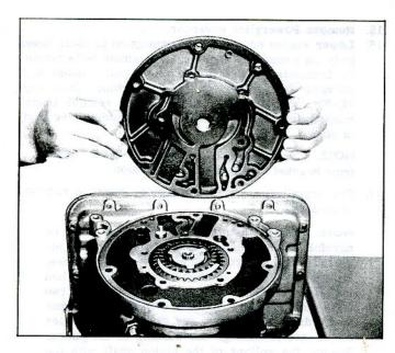
Fig. 7E-59—Installing Front Pump Cover
