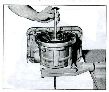
Fig. 7E-58-Installing Front Pump Drive Shaft
