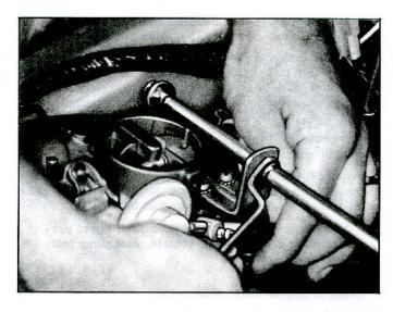
Fig. 9-Adjusting Accelerator Rod
