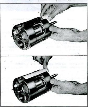
Fig. 54-Installing Suction Crossover Cover
