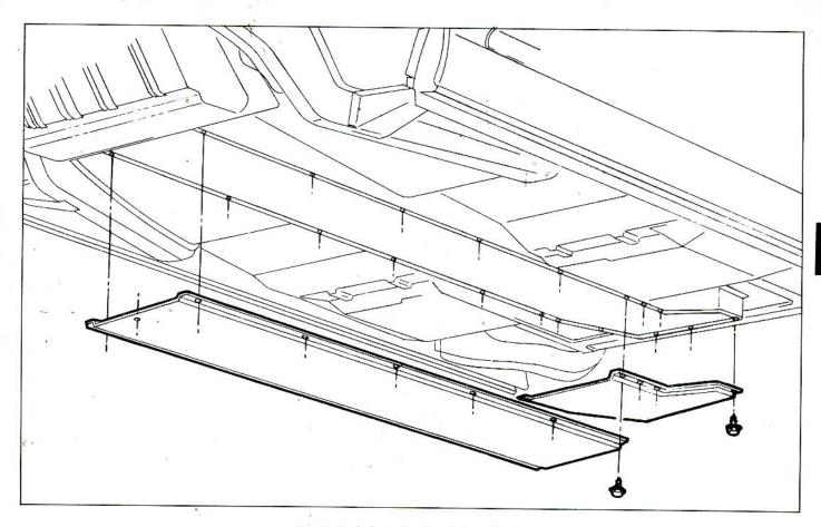
Fig. 2—Underbody Front and Rear Shields
