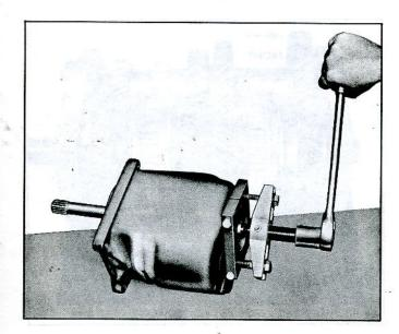
Fig. 7B-5-Removing Clutch Gear Bearing with Puller J-8880
