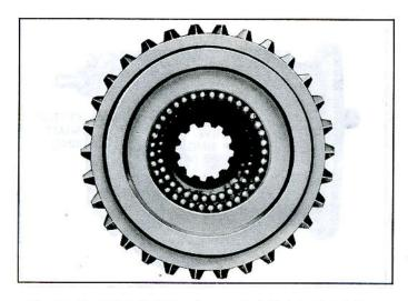
Fig. 7B-15-Mainshaft Roller Bearings Installed in Clutch Gear
