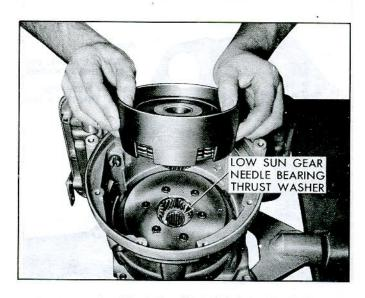
Fig. 7E-54-Installing Clutch Drum
