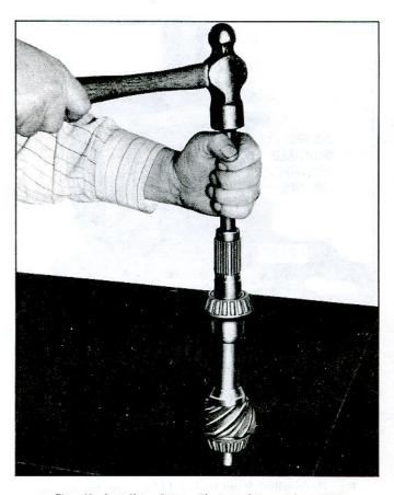
Fig. 41-Installing Pinion Shaft Bushing with J-8333
