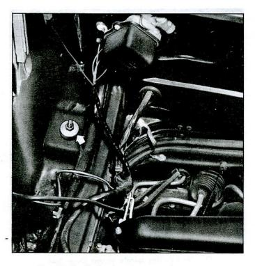
Fig. 75-Shock Absorber Upper Attachment Location
