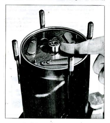
Fig. 44-Proper Oil Pump Gear Positioning
