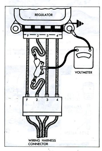
Fig. 10c-Checking Field Relay
