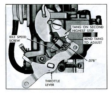
Fig. 12-Fast Idle Cam Adjustment
