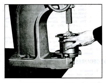
Fig. 41-Pressing Turbine Shaft from Impeller
