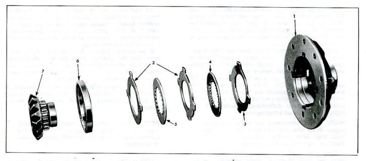
Fig. 54—Positraction Differential—Exploded View
