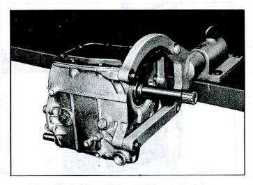
Fig. 7A-4-Transmission in Fixture J-7896
