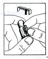
Fig. 15—Inserting Spring
