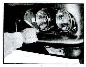
Fig. 10-Removing Retaining Ring Spring
