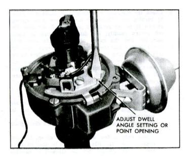
Fig. 2-Point Adjustment
