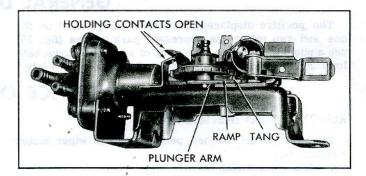
Fig. 39-Releasing Pump from Lockout Position
