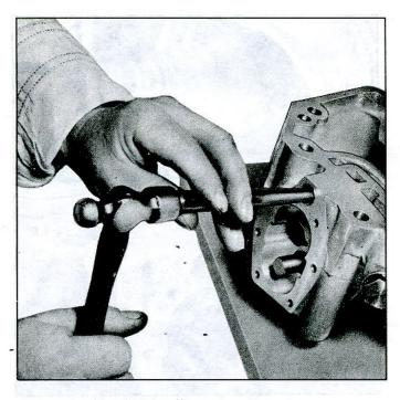
Fig. 117-Installing Oil Gallery Plugs
