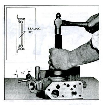
Fig. 114-Installing Rear Housing Seal
