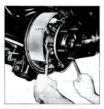
Fig. 65-Removing Wheel Drive Spindle
