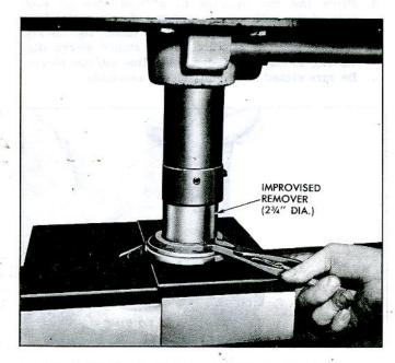
Fig. 7B-12-Pressing Rear Bearing from Bearing Retainer
