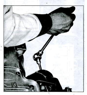
Fig. 51-Removing Left Front Shroud
