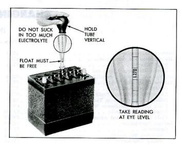
Fig. 2b—Testing Specific Gravity of Battery
