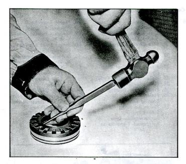
Fig. 22—Removing Pinion Front Bearing Race from Pinion Adjusting Sleeve
