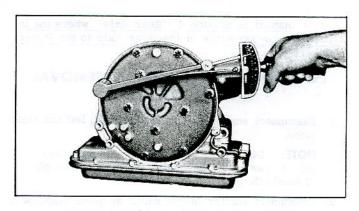
Fig. 7E-61-Measuring Front Pump Bolt Torque
