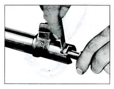
Fig. 16-Checking Lash Adjuster End Clearance
