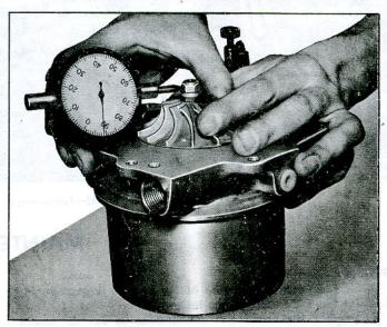
Fig. 38-Gauging Turbine Shaft Radial Play
