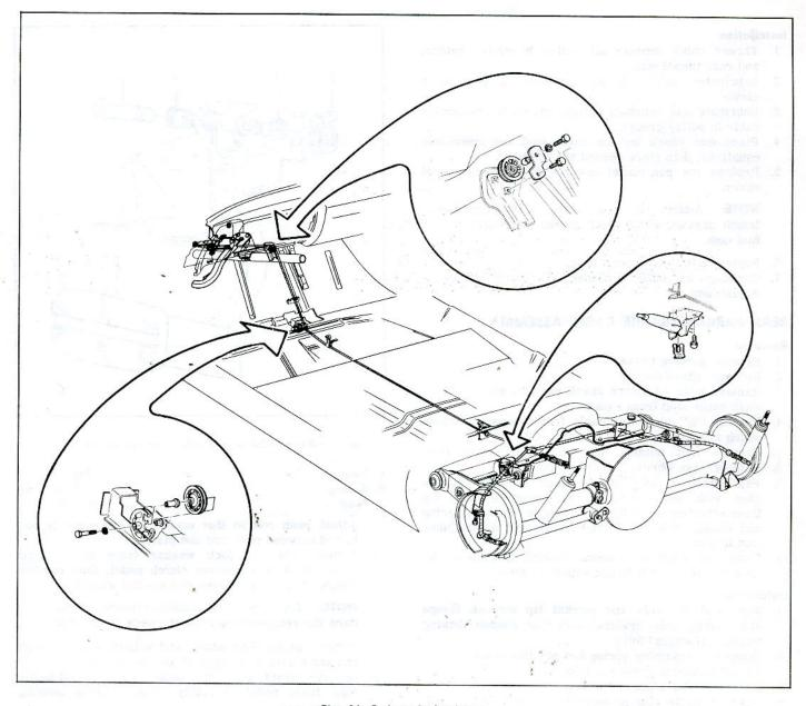
Fig. 16-Parking Brake System
