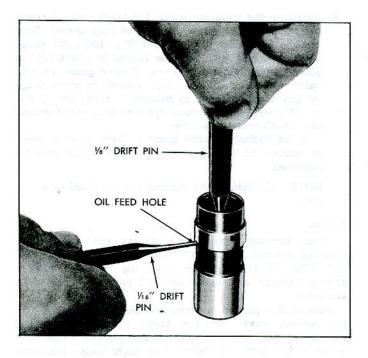
Fig. 96-Assembling the Hydraulic Lifter
