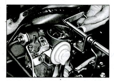
Fig. 8-Adjusting Throttle Rod
