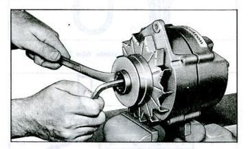
Fig. 14c-Pulley Removal
