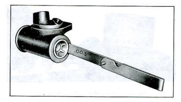
Fig. 25-Checking Wheel Cylinder Piston Fit
