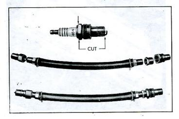
Fig. 37-Air Adapter Tool
