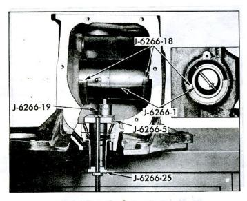
Fig. 19—Pinion Depth Shim Selection Gauge—Installed Views
