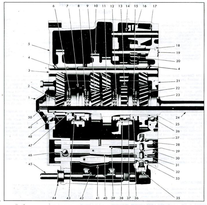
Fig. 7B-1-Corvair Four-Speed Transmission-Cross Sectional View
