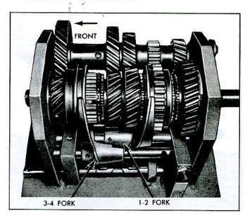
Fig. 7B-3-Shift Forks Installed
