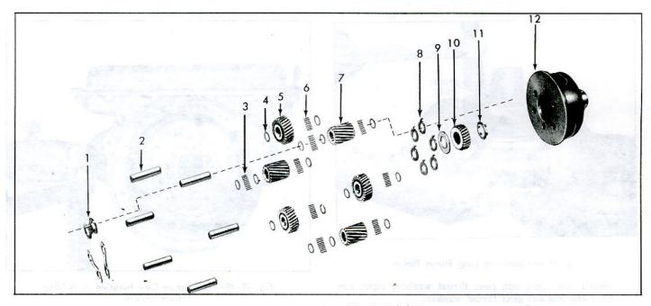
Fig. 7E-45-Planet Carrier Assembly-Exploded View
