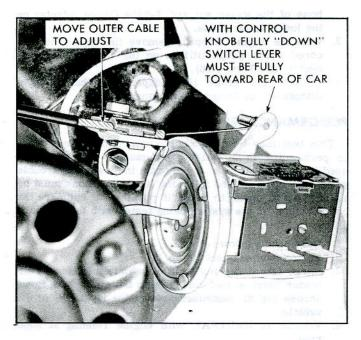
Fig. 17—Thermostatic Switch Cable Adjustment
