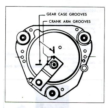
Fig. 35-Wiper Crank Arm in Park Position
