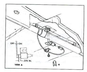
Fig. 17—Backing Lamp Switch—3-Speed Transmission
